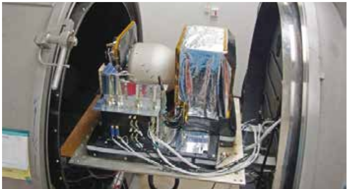
The Microwave Humidity Sounder (MHS) instrument of Metop-C is fitted with sensors and measurement cables and put into the chamber for thermal vacuum testing (source: Airbus Defence and Space)
