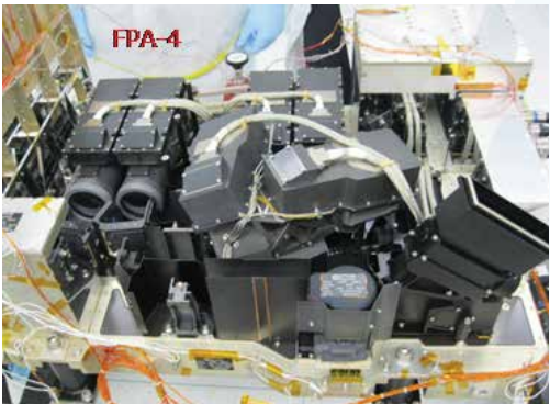
Dismounting of the GOME-2 instrument at Leonardo premises, for the repair of one focal plane assembly (marked FPA4)
