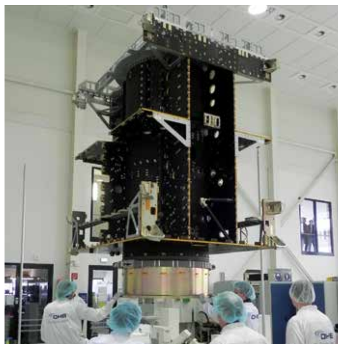
Optical bench of the Flexible Combined Imager (above) and MTG platform structural/thermal model at industry premises (right)
