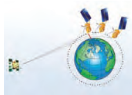
Principle of radio occultation measurements as used by the GRAS SAF. The red line is the vertical profile of meteorological products
