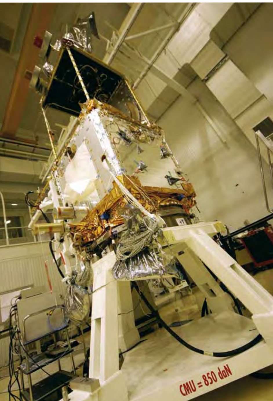
Jason-2 satellite in the cleanroom, being built (image: Yoann Obrenovitch)
