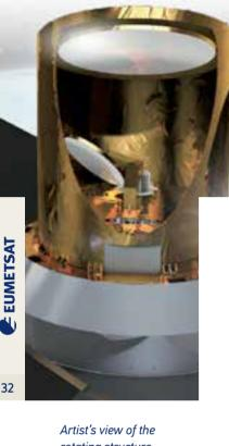
rotating structure of the new Microwave Imager (MWI) instrument to be flown on the Metop-SG B satellites to map precipitation (source: industry)
