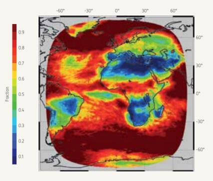
Monthly averaged CLAAS product for cloud fraction (CFC) with a latitudelongitude sampling of 0.05 degree (source: CM SAF) An undersampling strategy was tested and adopted to speed up the reprocessing of MSG products by a factor of ~2.5, while fulfilling the needs of reanalysis projects. Thus, more than two years of MSG wind vector and radiance products have already been reprocessed, including the full year 2008, and the full Climate Data Record will become available by mid-2014.
