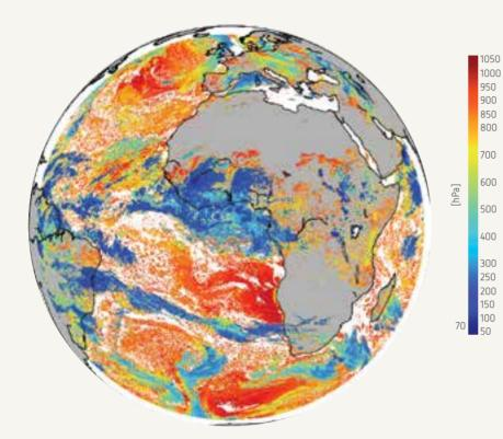
Cloud Top Pressure (hPa) as determined by the Optimal Cloud Analysis algorithm
