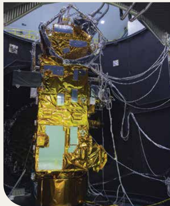
Metop-C's service module undergoes thermal vacuum tests in March 2017 (source: ESA, G. Porter)
