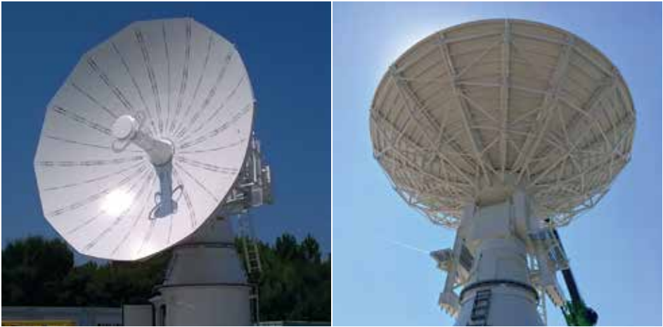
Ka-band mission data acquisition antenna (left) and S-band telemetry tracking and control antenna (right) under factory acceptance testing before shipment to Svalbard
