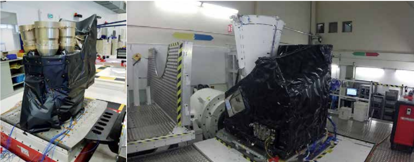
Structural and thermal models of the LI (left) and FCI (right) of MTG-I (source: Thales Alenia Space, OHB, ESA)
