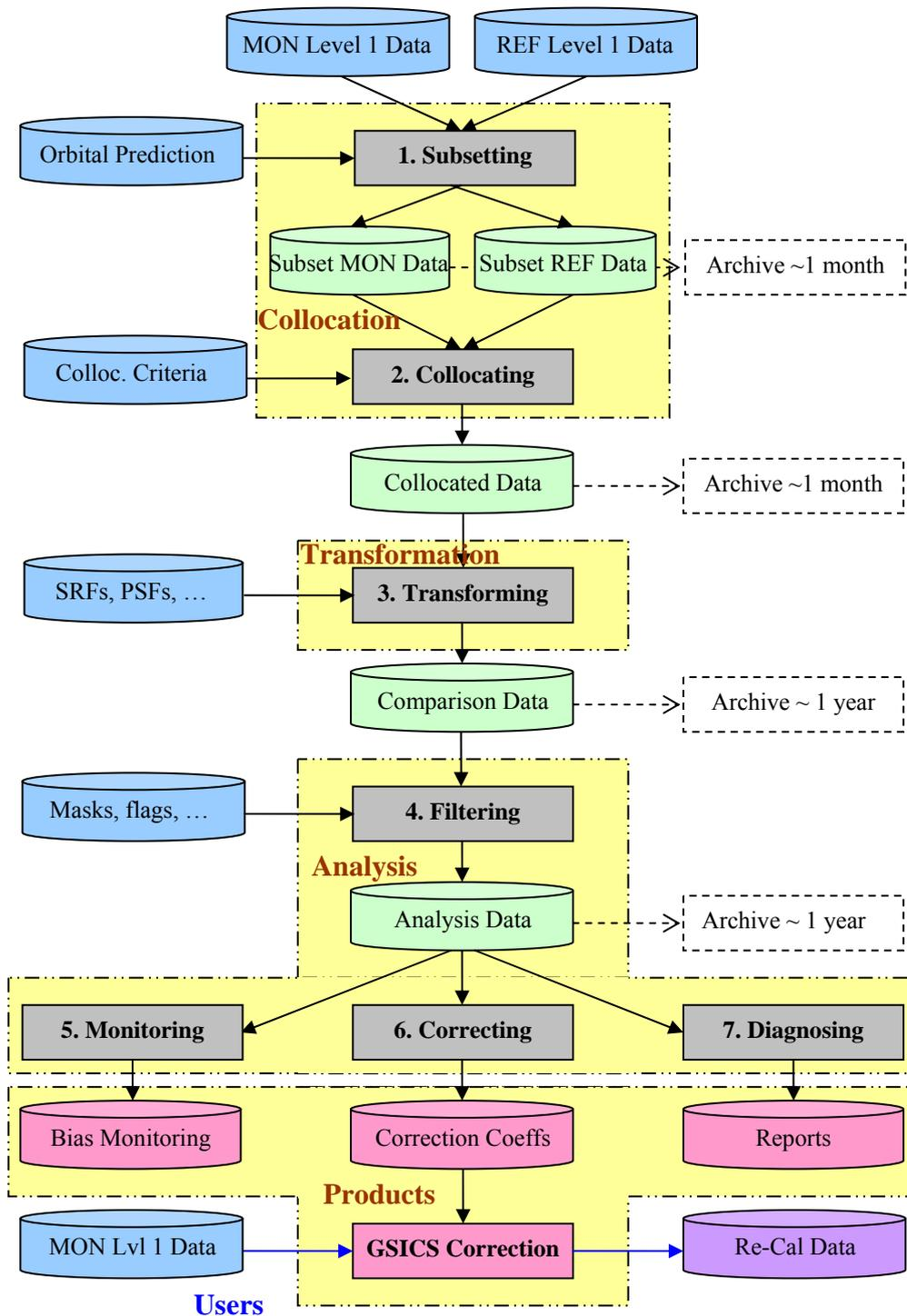
*Figure 1: Diagram of generic data flow for inter-calibration of monitored (MON) instrument with respect to reference (REF) instrument*
