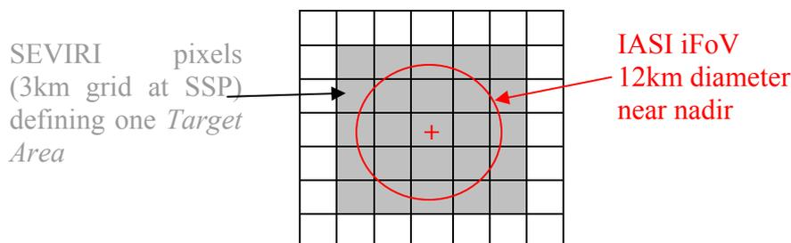
**Figure 8: Definition of Target Area as 5x5 SEVIRI pixels to spatially match an IASI iFoV.**
