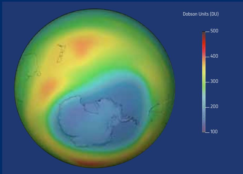
Also very important is GOME-2's capacity to significantly extend the long time series of measurements already gathered by GOME-1, which will help continue the monitoring of ozone depletion.
