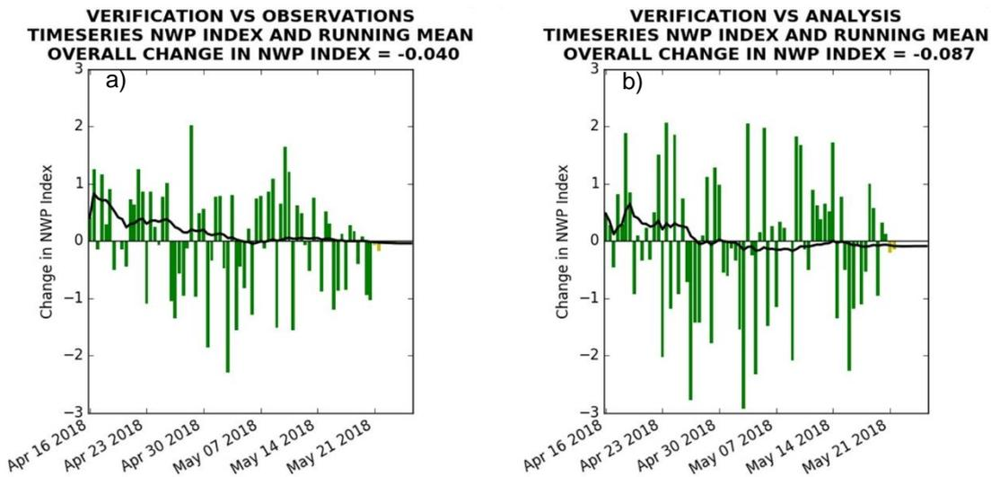
Figure 4. Global NWP index changes between +SLSTR and control (+SLSTR minus control) when compared against a) observations and b) analyses during 15 April – 21 May 2018.
