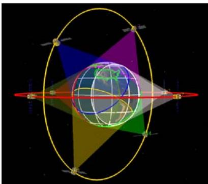
**Figure 1. Equatorial-Polar (EP) Constellation**
