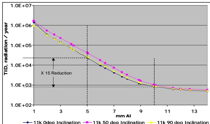
Figure 5. TID attenuation vs. aluminum (Al) shielding
