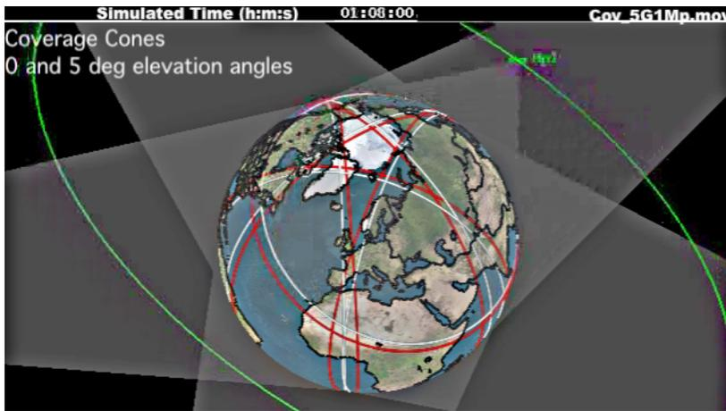
**Figure 7. Coverage from a single MEO satellite complementing the International Geosynchronous satellite systems. Elevation angles are shown for 0 degrees (red) and 5 degrees (white).**
