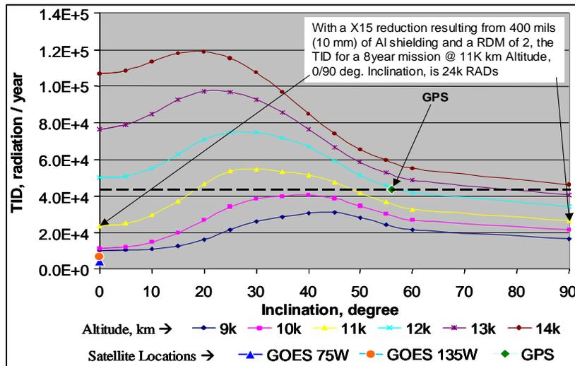
Figure 4. Annual TID received by a silicon chip with 5mm aluminum shielding (calculations based on solar maximum conditions).
