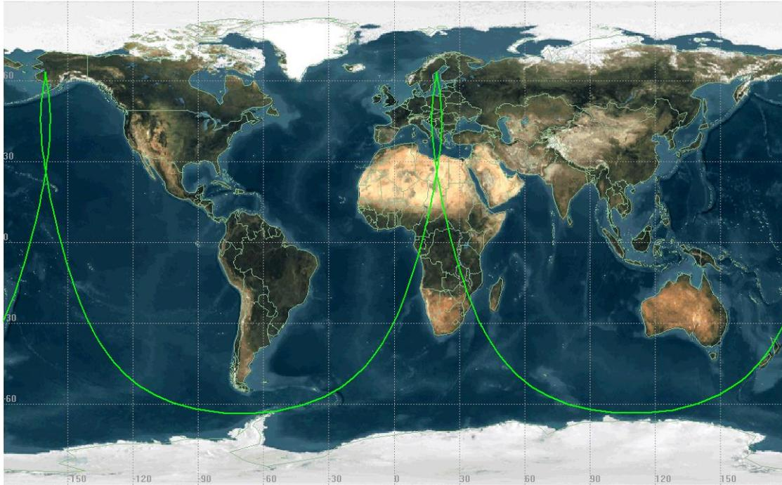
Figure 2. Example ground track of a Molniya orbit satellite. The satellite will alternate between the two apogee points in the respective cusps of the orbital track. Any ground station N of 60 degrees N will be able to see the satellite during the entirety of both apogee dwell periods.
