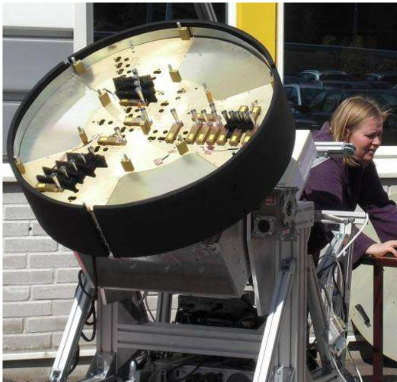
Figure 4: The demonstrator with its 20 antenna elements and rotating structure.
