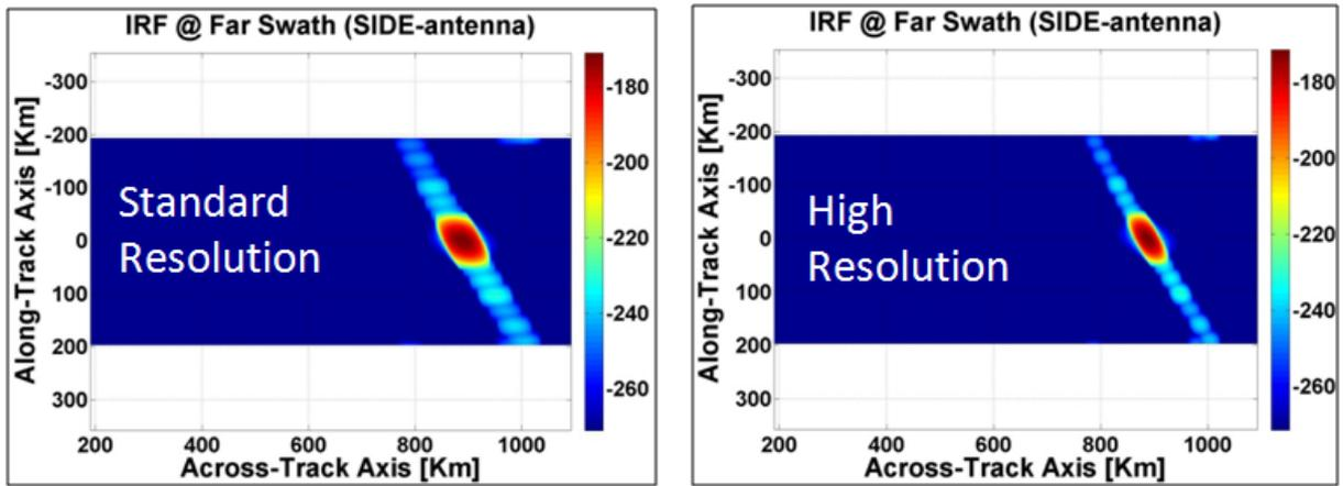
Figure 6: Comparison between the Impulse Response Function of the standard and high-resolution product.
