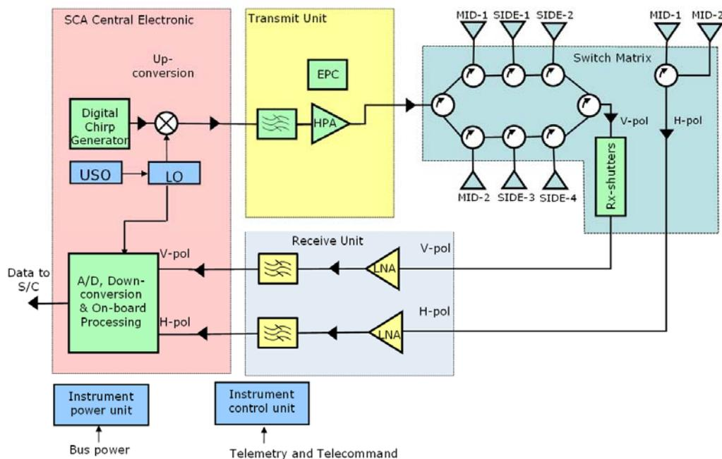
**Figure 2:** SCA instrument block diagram for the case of simultaneous acquisition of V and H-polarized signals from the mid antennas.
