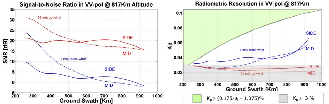
Figure 4: On the left side: Signal-to-Noise Ratio in VV-polarisation for the MID and SIDE antennas in case of 25 m/s up-wind (red lines) and 4 m/s cross-wind (blue lines). On the right side: radiometric resolution performance versus requirements in VV-polarisation.
