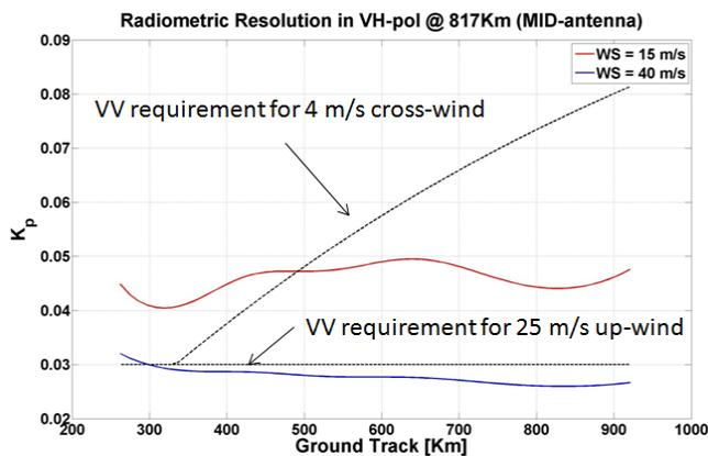
Figure 8: Radiometric resolution in VH-pol for the case of 15 m/s and 40 m/s wind speed.
