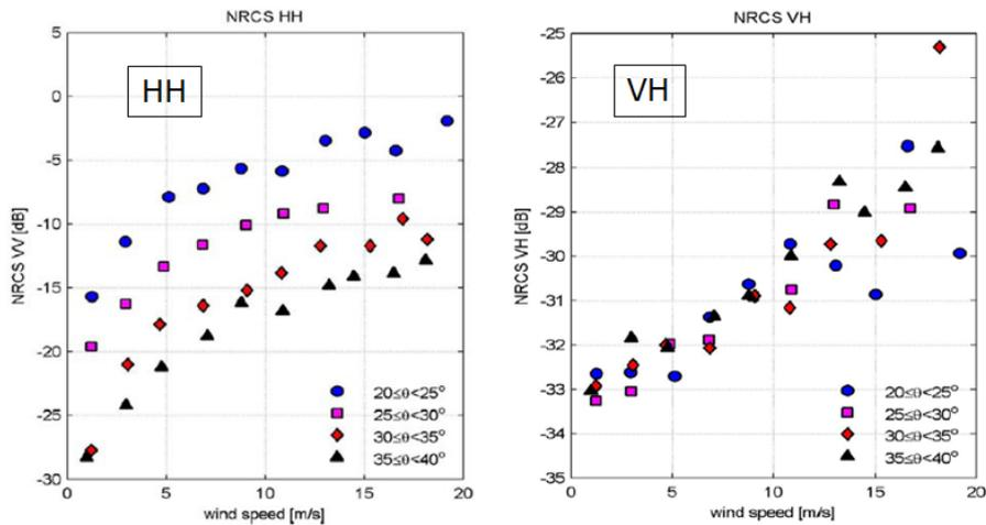
Figure 7: Normalised radar cross section versus wind speed in HH and VH polarisation.
