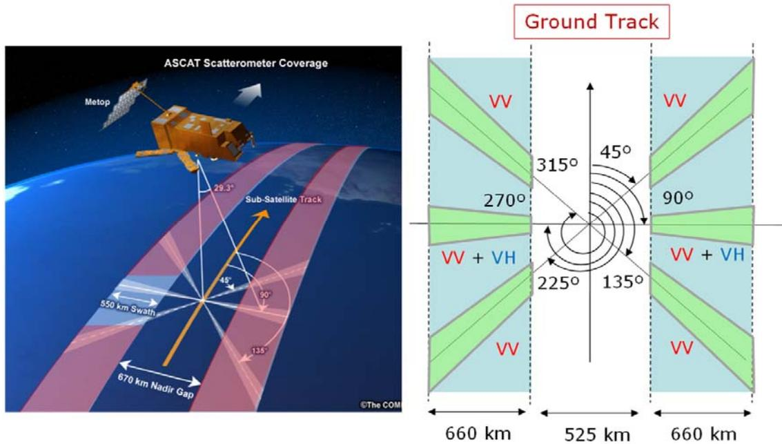
Figure 1: ASCAT measurement geometry (left) versus SCA measurement geometry (right)
