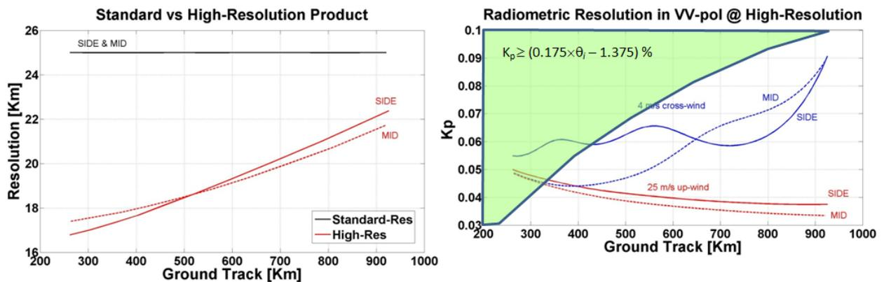
Figure 5: Standard versus high resolution product (left); Radiometric Resolution of the high resolution product in VV-polarisation (right).
