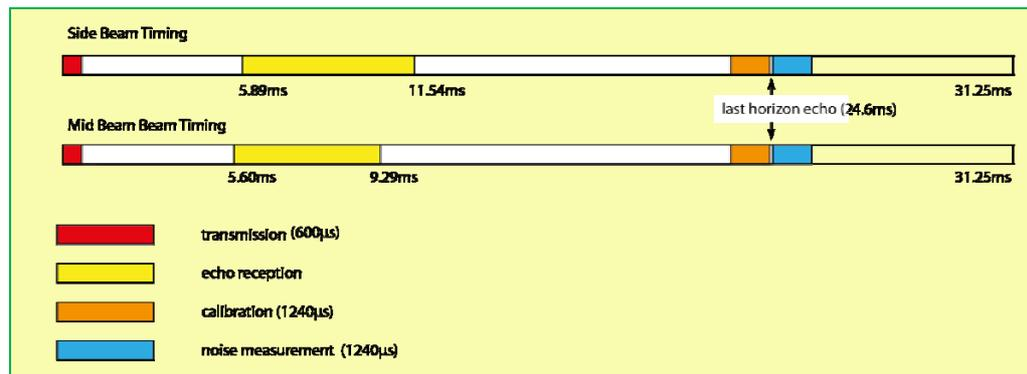
Figure 8: SCA Instrument Timing
