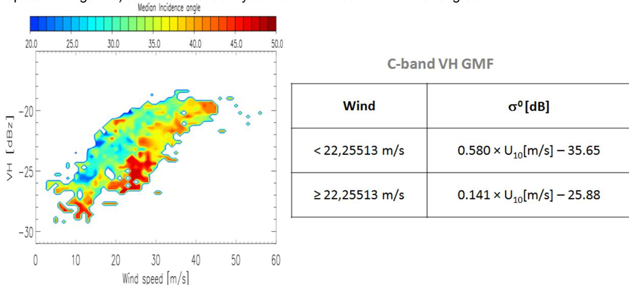
**Figure 3: Radarsat-2 versus NOAA SFMR (left); VH-pol Geophysical Model Function (right)**
