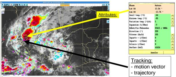
Figure 1: RDT as visualized by Météo-France forecasters with SYNERGIE workstation. Background image: enhanced 10.8µm satellite-image. Convective cell is characterized by various attributes and its trajectory.
