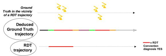
Figure 4: Validation outline. The electrical-trajectory (ground truth trajectory) is built with the strokes in the vicinity of a RDT trajectory (upper part of the figure). Some sections are then defined for deduced ground truth trajectory (middle part). The RDT convection diagnosis (lower part) is compared to electrical observed ground truth.
