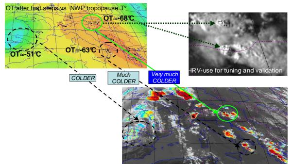
Figure 2: Tropopause-temperature-diagnosis helps to eliminate wrong OT detected after first steps, rejected OT have a temperature not cold enough compared tropopause. High Resolution visible Image confirms the OT.
