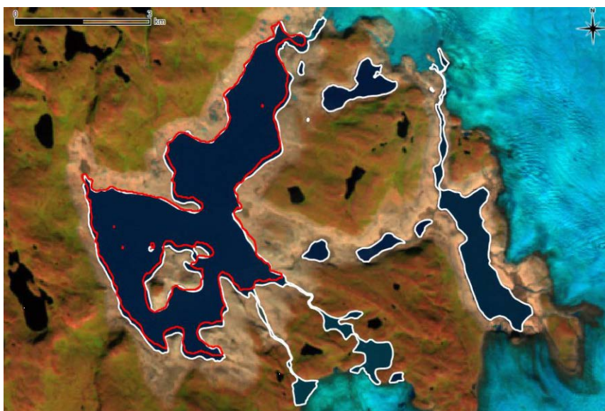
Figure 5.2: Comparison of outlines of glacier Lake Tininnilik, West-Greenland, derived from Landsat 7 ETM+ scene of 2010-08-17 (white outlines) and an Envisat ASAR scene of 2010-08-15 (red outlines). A RGB composite of the Landsat 7 ETM+ scene is used as background.
