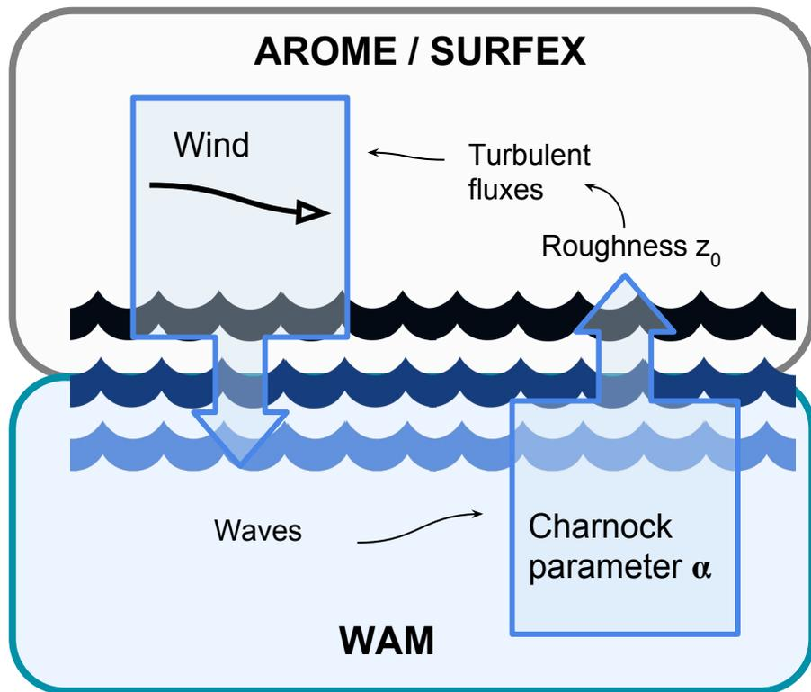
1. The surface roughness  $z_0$  over open sea depends on the Charnock's parameter  $\alpha$
