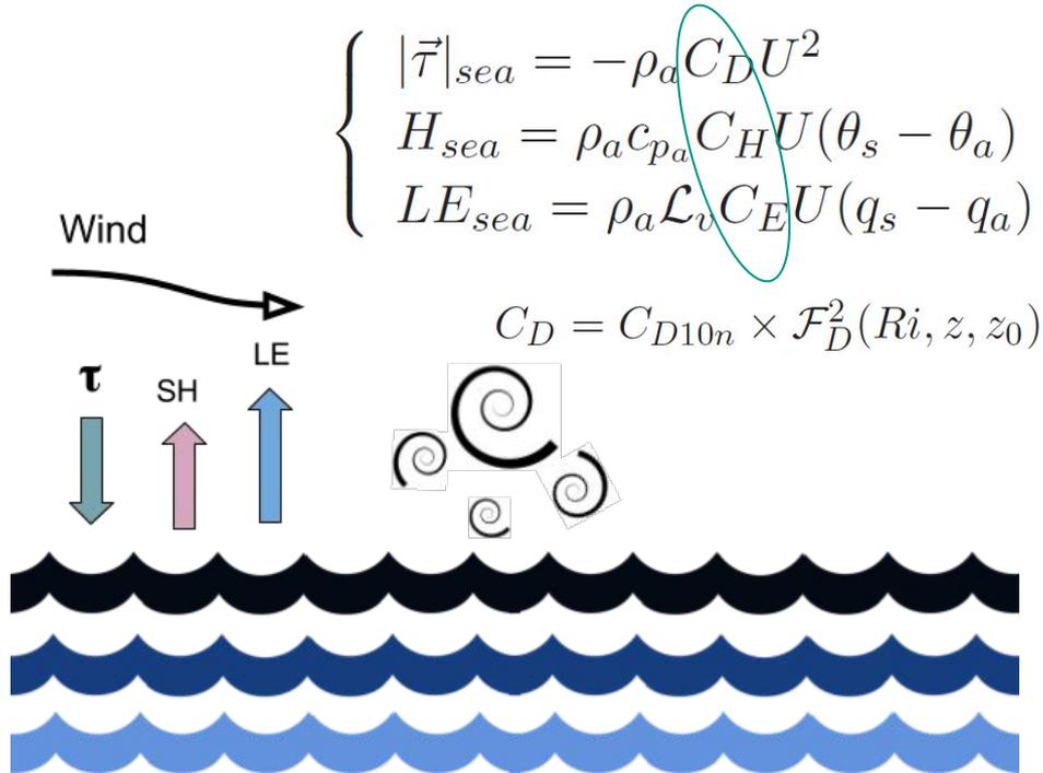
1. Turbulent fluxes from the mean meteorological gradients with the use of transfer coefficients  $C_D$ ,  $C_H$  and  $C_E$
