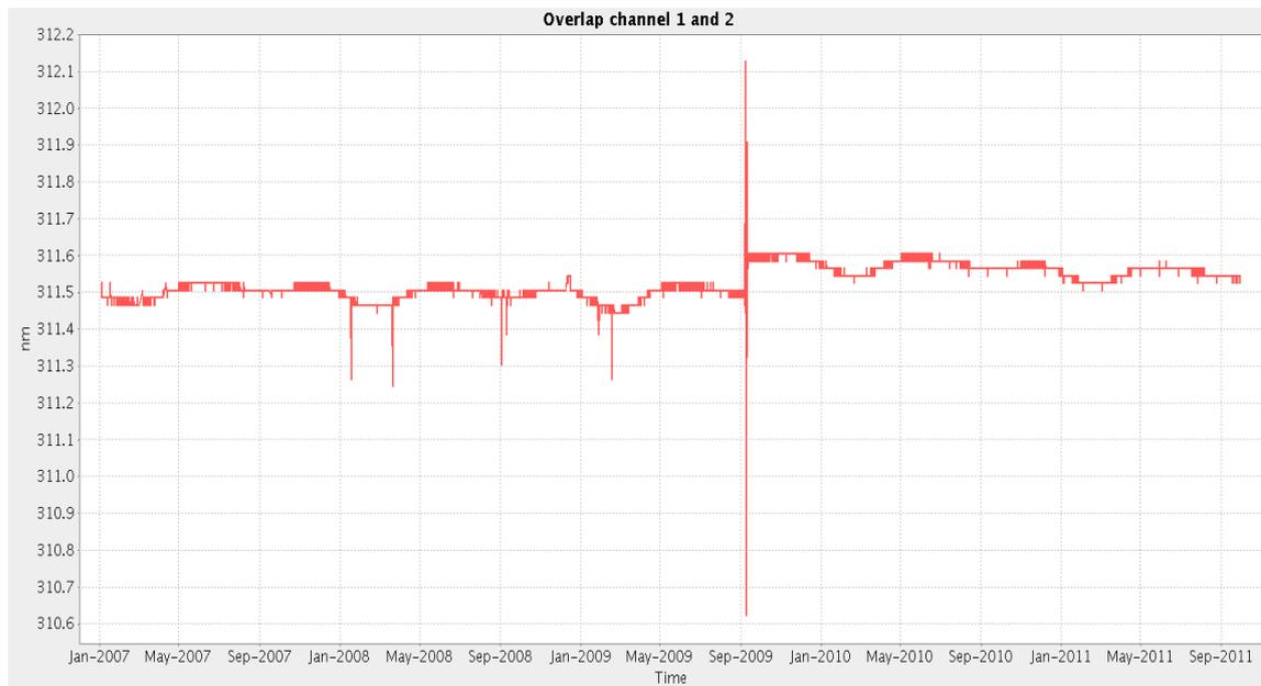
Figure 25: Overlap-point position for the transition between channel 1 and 2 in wavelength space
