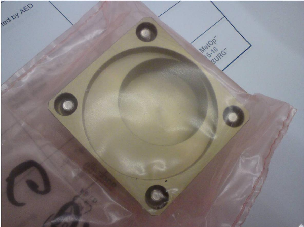
Fig. 7.1.4: Cap covering the flange of the evacuation system during launch and in orbit
