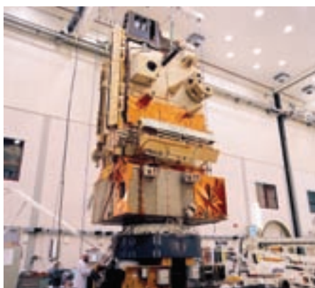
The Metop structural model undergoing tests
