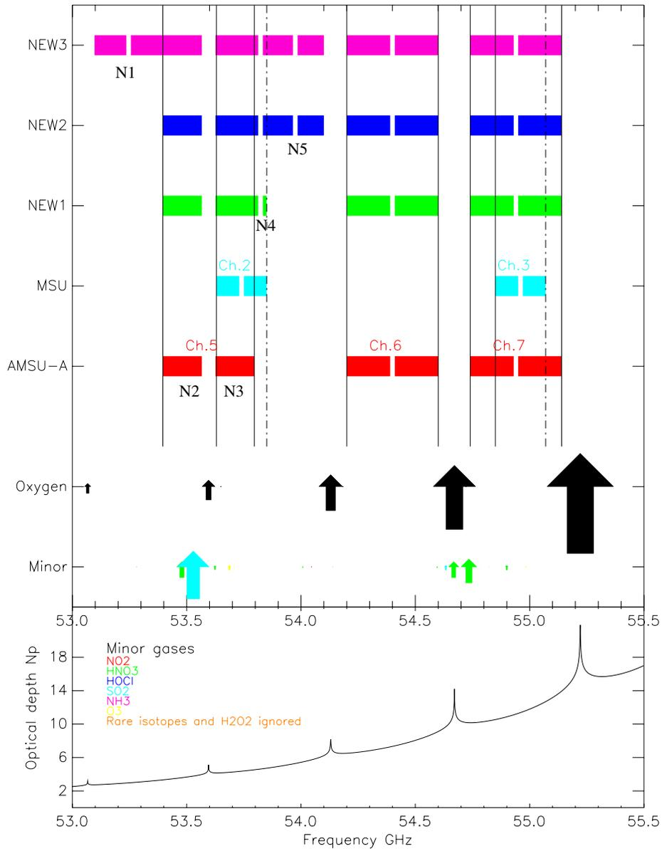
Figure 9: Comparison of MSU, AMSU and proposed channel configurations with oxygen and minor gas spectroscopic features.
