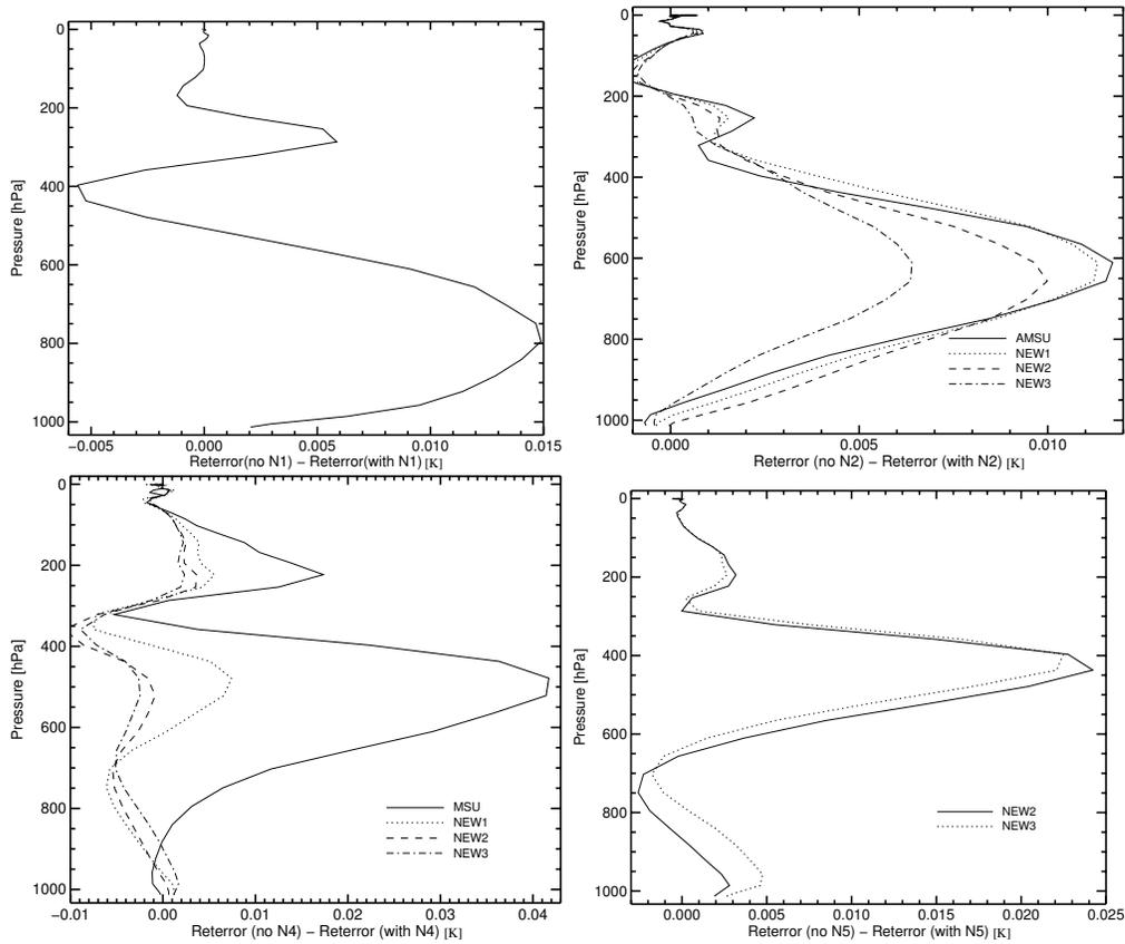
Figure 12: Top left: Impact of channel N1, Top right: Impact of channel N2, Bottom Left: Impact of channel N4, Bottom right: Impact of channel N5. All plots are for viewing angle  $30^\circ$ .
