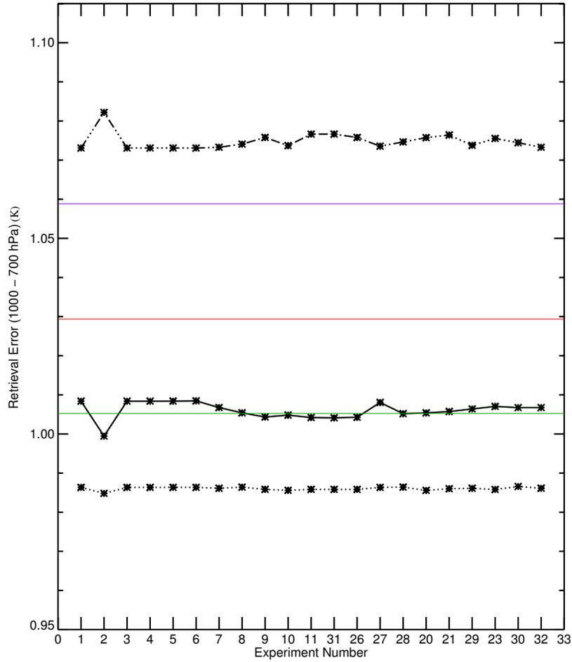
Figure 3: Layer averaged (1000 to 700 hPa) temperature retrieval error for experiments listed in Tables 2 and 3. The dotted line is for viewing angle  $10^\circ$ , solid line for  $30^\circ$  and dash-dotted line for  $50^\circ$ . The horizontal green line shows the retrieval error if channel 3 is removed from the analysis, red line if channel 4 is removed and purple when channel 5 is removed. The polarisations of other channels remain the same as in experiments 6 or 7.
