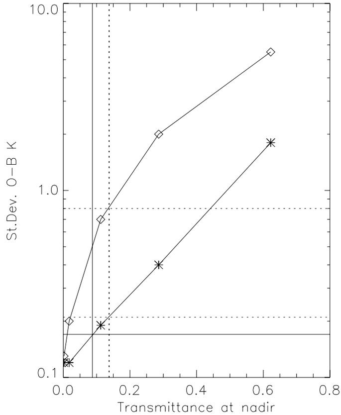
Figure 7: Relationship of mis-fit of AMSU observations to surface to space transmittance for sea points (asterisk) and land points (diamonds). The vertical continuous and dotted line show the surface to space transmittance for the lower frequency side band of AMSU channel 5 and the higher frequency sideband respectively (almost equivalent to MSU channel 2). The horizontal continuous and dotted lines show the corresponding expected values of the standard deviation of O-B.
