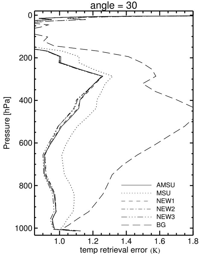
Figure 10: Temperature retrieval errors for the new instruments.
