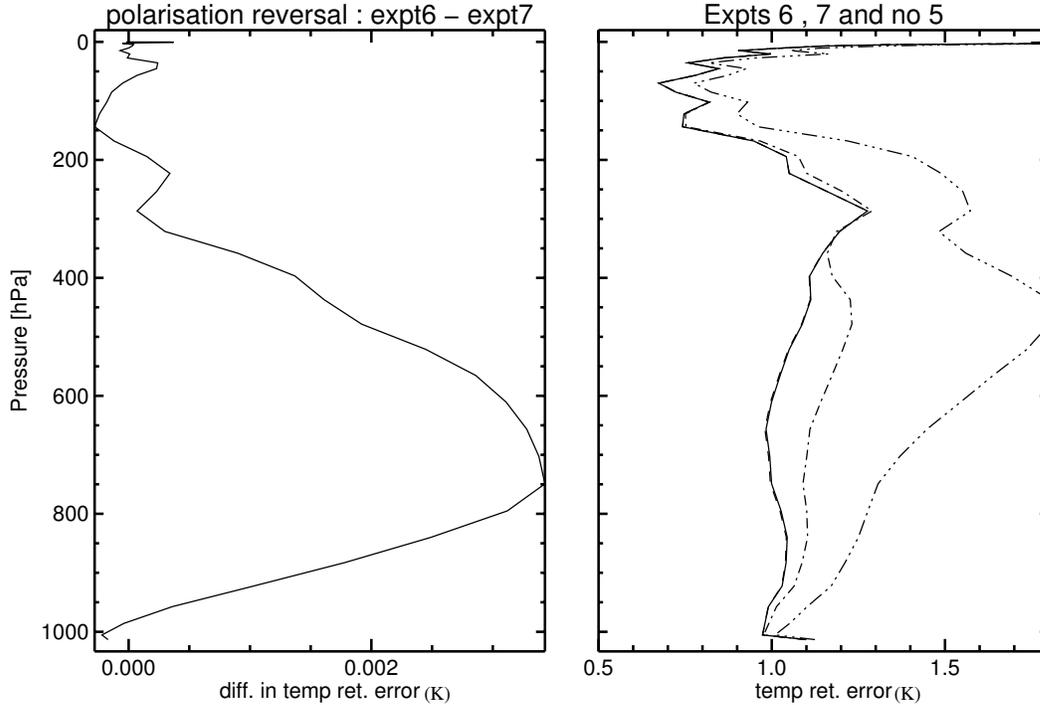
Figure 4: The right panel shows temperature retrieval error for experiments 6 where channel 5 is in QV polarisation (solid), experiment 7 where channel 5 is in QH polarisation (dashed) and when channel 5 is removed (dash-dotted) at a viewing angle of  $30^\circ$ . The dash-dot-dot-dotted line shows the background error. The left panel shows the difference between experiments 6 and 7.
