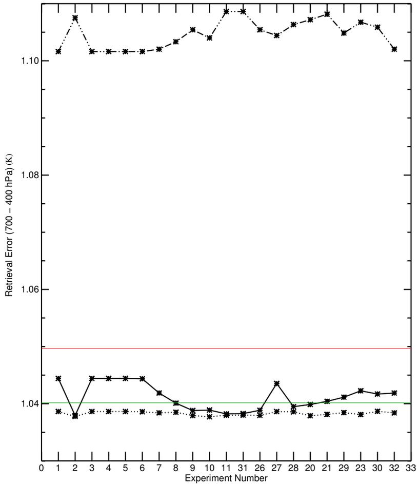
Figure 2: Layer averaged (700 to 400 hPa) temperature retrieval error (in K) for experiments listed in Tables 2 and 3. The dotted line is for viewing angle  $10^\circ$ , solid line for  $30^\circ$  and dash-dotted line for  $50^\circ$ . The horizontal green line shows the retrieval error at  $30^\circ$  when channel 3 is removed from the analysis and red line when channel 4 is removed. When channel 5 is removed, the retrieval error is about 1.17.
