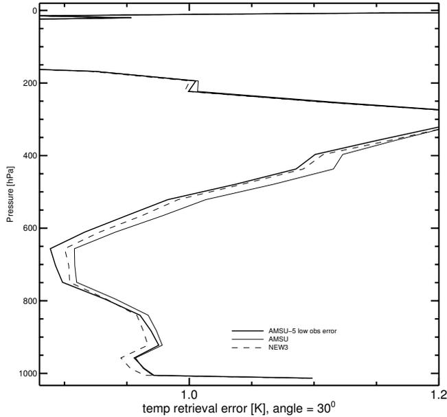
Figure 13: Temperature retrieval errors for AMSU-A (solid) and NEW3 (dashed). The thick and lines respectively represent cases with low and high observation error for channel 5.
