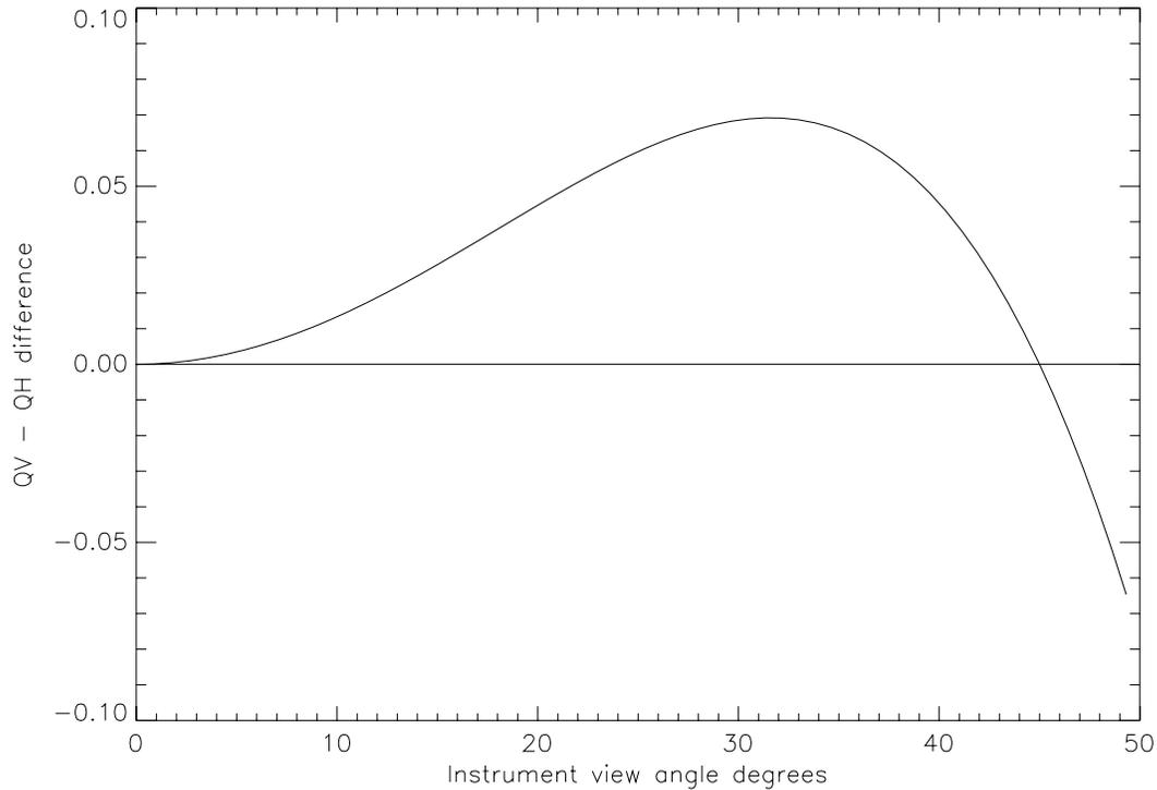
Figure 1: Emissivity difference in QV and QH for a highly polarised flat smooth surface (permittivity 10-8i).
