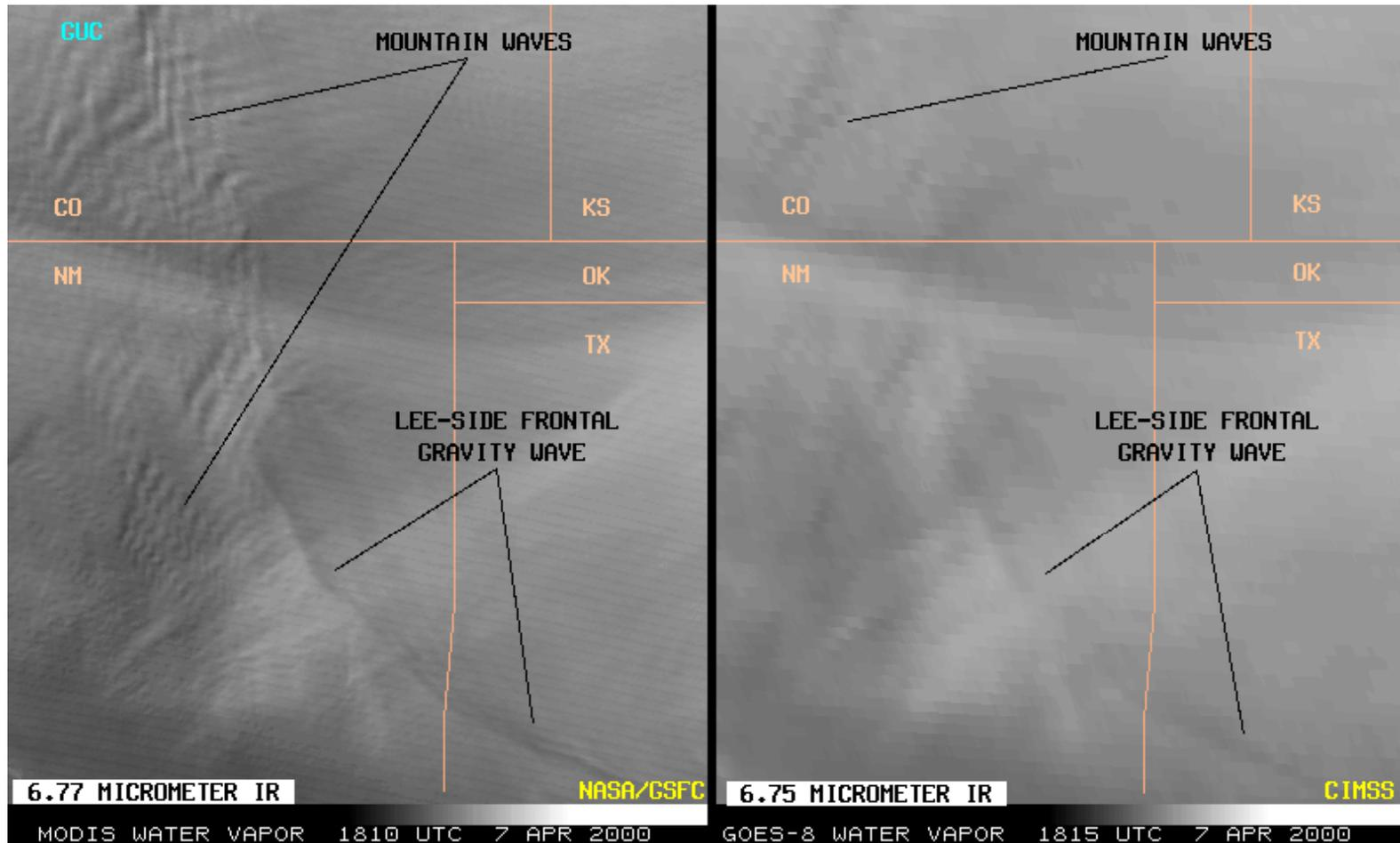
MODIS has 1km water vapor band compared to 8km of GOES
