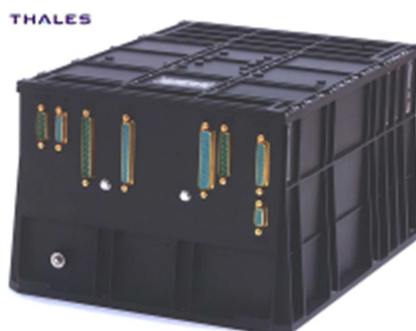
Figure 10 : SARAL ARGOS-3 reception instrument
