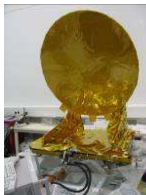
Figure 5 : SARAL/AltiKa radiometer Instrument and antenna (shared with altimeter)
