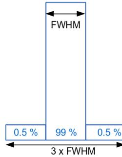
Figure 4.1.1: Modelled ISRF shape for the VII-5 channel.
