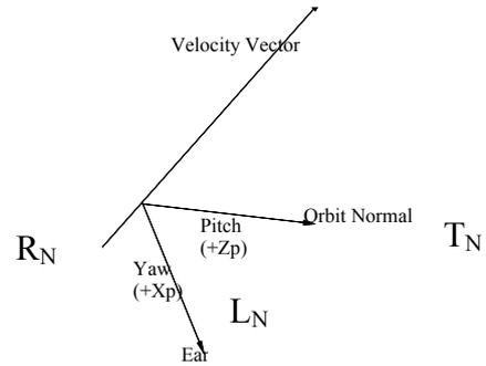
The above-mentioned definitions are those followed by NOAA. The conversions between the NOAA local orbital Reference Frame [ $T_N R_N L_N$ ] and the [ $T, R, L$ ] frame used in the EPS Programme are given below (the “x” symbol denotes the cross-product operand):
