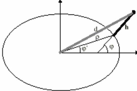
Figure 2: Geodetic position
