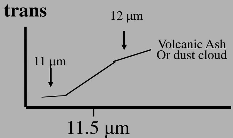
If 12 μm sees considerably higher BT than 11 μm then the atmosphere probably contains dust (as above) or volcanic ash; if 11 μm sees the same or higher BT than 12 μm the atmosphere viewed does not contain dust cloud or volcanic ash;
