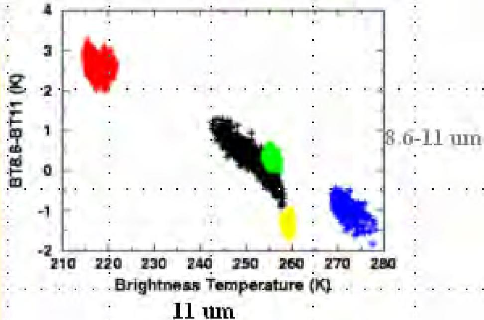
These three scatter plots illustrate how different types of clouds, snow and clear ground have different spectral signatures when plotted against 11  $\mu$  brightness temperature.
