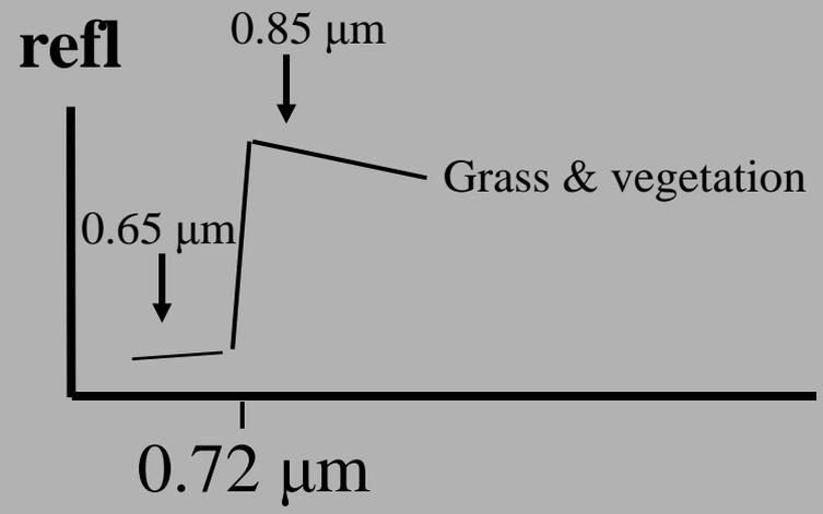
If 0.65 μm and 0.85 μm channels see the same reflectance then surface viewed is not vegetation;
