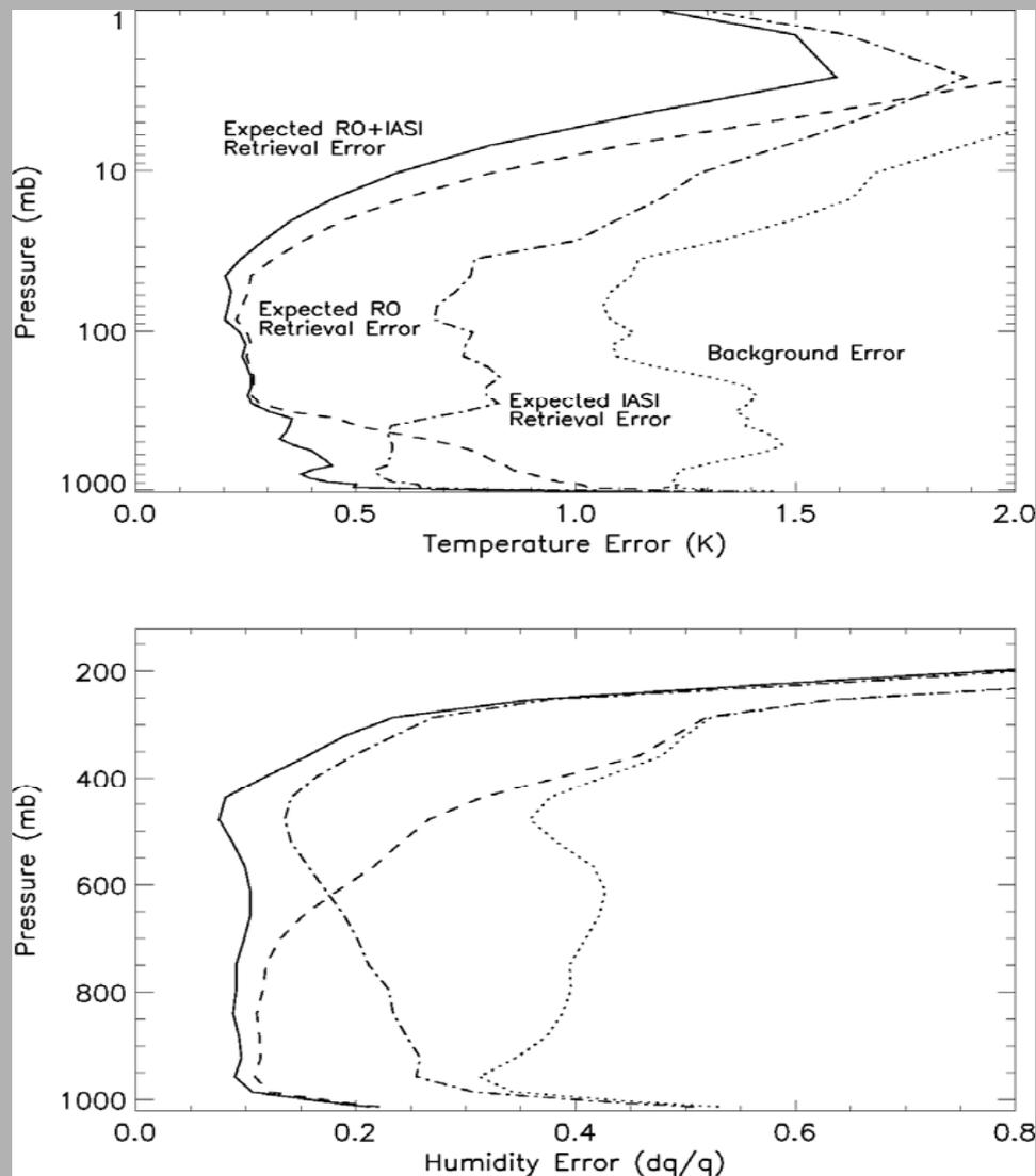
The figure at the left is From Collard and Healy (2003) showing the anticipated accuracy when GPS and hyperspectral sounding data are combined. Notice that by utilizing the two together that the answer is better than either separately.
