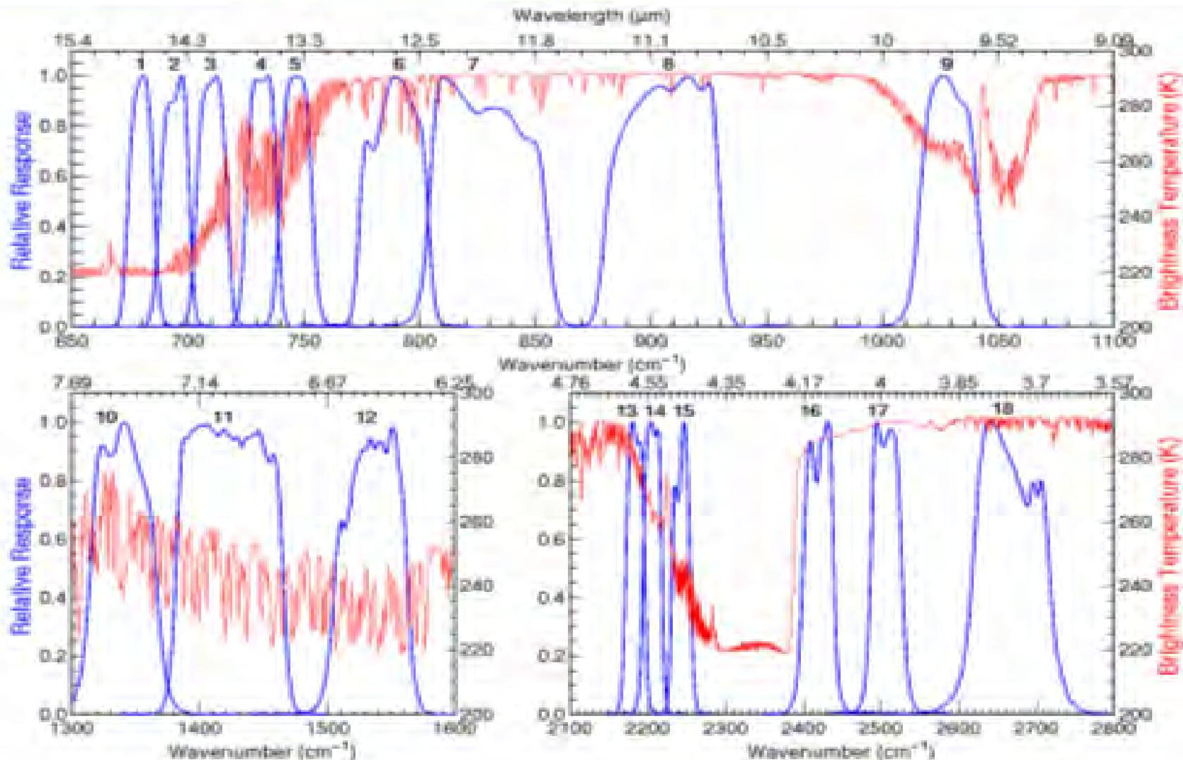
The red curve shows the thermal terrestrial spectrum between 4 μm and 15 μm in terms of brightness temperatures at the top of the atmosphere calculated for a standard mid-latitude summer atmosphere and nadir view. The blue curves depict the relative spectral response functions of the GOES I-M series sounder instrument.
