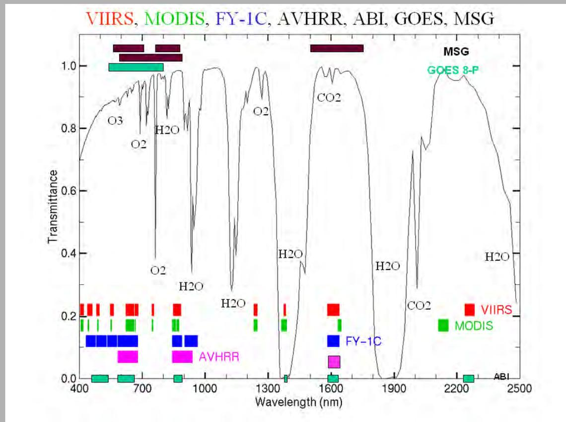
**One might ask “why the various satellite imager channel widths and spectral locations?” The answers are complex, but basically relate back to the resolutions described earlier (Lecture A) and specifically the tradeoff between desired spectral resolutions versus the practicality of spatial resolution versus obtaining a high enough signal to noise ratio so that the instrument’s data may be used to describe the feature of interest to a desired accuracy level**
