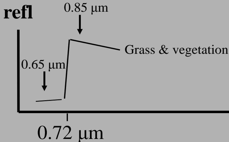
If 0.65  $\mu\text{m}$  and 0.85  $\mu\text{m}$  channels see the same reflectance then surface viewed is not vegetation;
