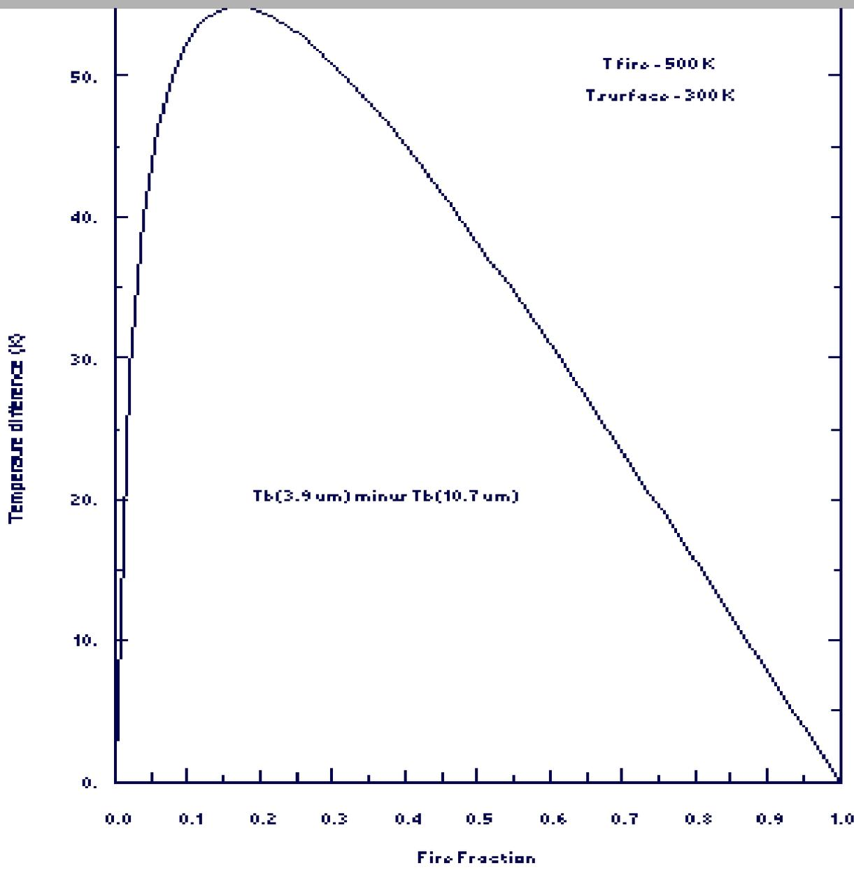
On the left is an example of the difference in temperature measured at 3.9 and 10.7 microns for a partially filled field of view (FOV) for nighttime when there is no solar reflection. In this example, the hot-area is at 500 K and the remainder of the pixel is at 300 K.
