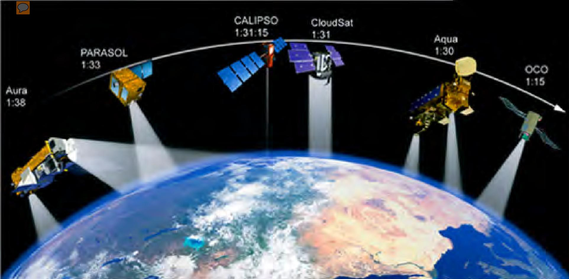
The “A Train” formation with equator crossing times. In the formation, the satellites nominally all trace out the same ground track. Click on the bottom right to see an animation of clouds made from the formation of Terra, SAC-C and LandSat-7 (an total interval of about 40 minutes from first to last).
