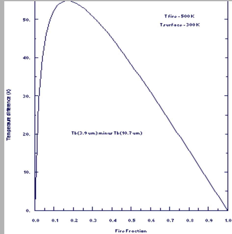
Response of 3.9 vs. 10.7 microns to Temperature variability in a FOV
