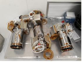
$\label{eq:control} Thermal \mbox{ model optical channels - courtesy Leonardo} \\ {\sf ESA \mbox{ UNCLASSIFIED - For Official Use} }$
