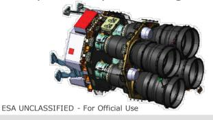
This brought many advantages (larger coverage while keeping fine spatial resolution and spectral performance, better configurability...) but it also means the field of view is more open to sun intrusions.
