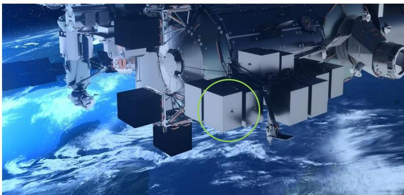
**Figure 6:** TOR on the Bartolomeo platform. The boxes indicate the envelope of instruments that can be accommodated.
