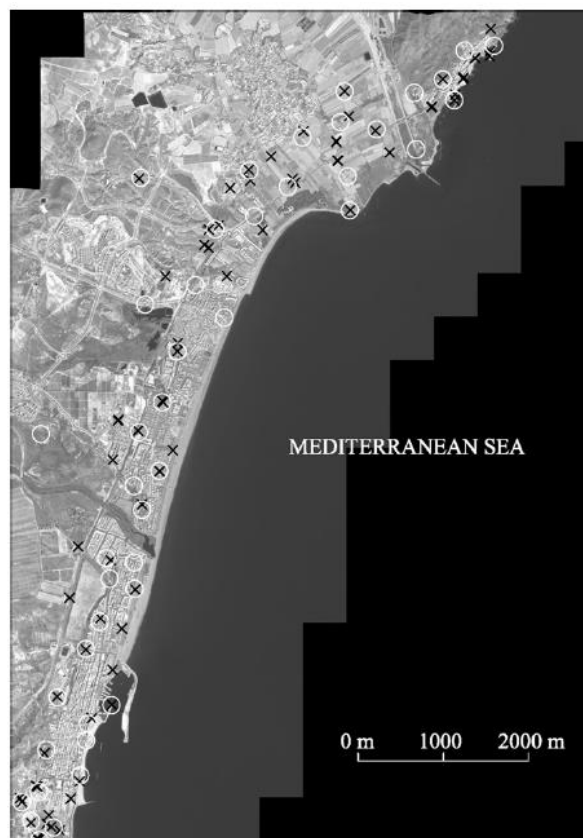
Figure 3-10: Distribution of 75 ICPs (black crosses) and 44 GCPs (white circles) overlaid on a GeoEye-1 panchromatic orthorectified image. (Aguilar et al. 2013)
