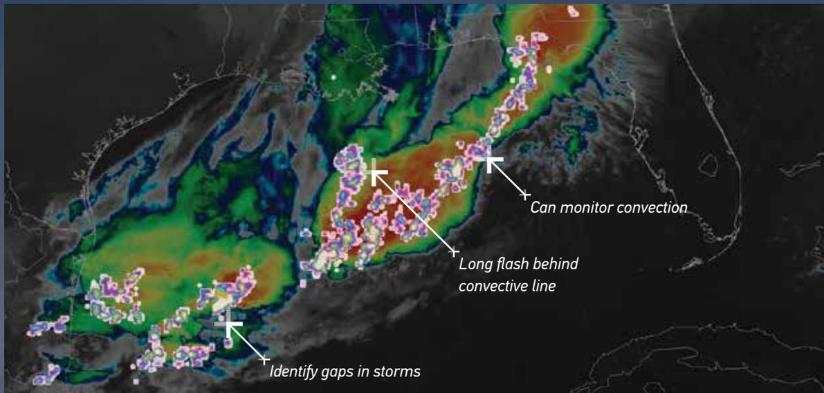
*This image taken by the US GOES Geostationary Lightning Mapper (GLM) instrument shows lightning activity in white-blue-magenta colours along a convective storm line (yellow-orange-red shades in background infrared imagery) over the Gulf of Mexico. The GOES GLM is a precursor to the MTG Lightning Imager.*
