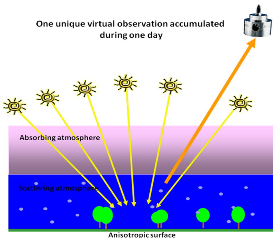
Figure 1: GSA Retrieval scheme. The observations accumulated during the day are used as an angular sampling of the surface.
