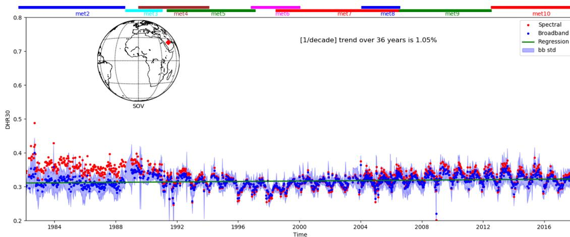
Figure 15: Time series of DHR30 (black-sky albedo) at site SOV (location shown in red on the map). The spectral albedo value is in red, the broadband albedo in blue (its standard deviation shaded blue) and the regression line for the trend in green. On the top of the plot, the available Meteosat satellites are indicated but only one (the operational) is used to construct the time series.
