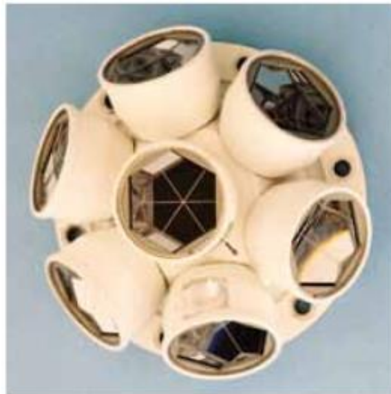
Figure 9: Photo of the Laser RetroReflector array
