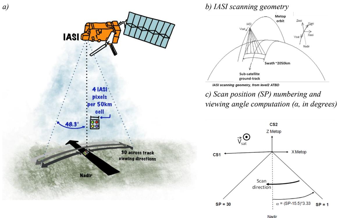
Figure 1: a) Idealised view of IASI sensing system. b) and c) IASI geometry from level 2 (EUMETSAT, 2020b).
