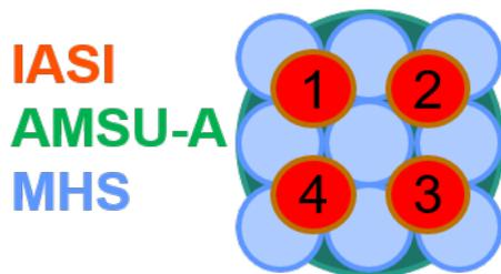
**Figure 3:** Idealised view of the IASI footprint geometry with the associated AMSU-A, MHS footprints. Each IASI field of view is composed of 4 IASI pixels, each IASI pixel diameter is approximatively 12km at nadir.
