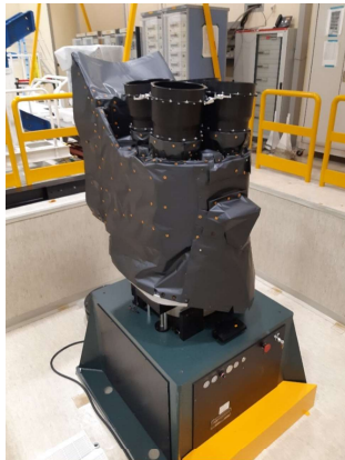
LOH PFM on the CoG measurement machine- courtesy Leonardo
