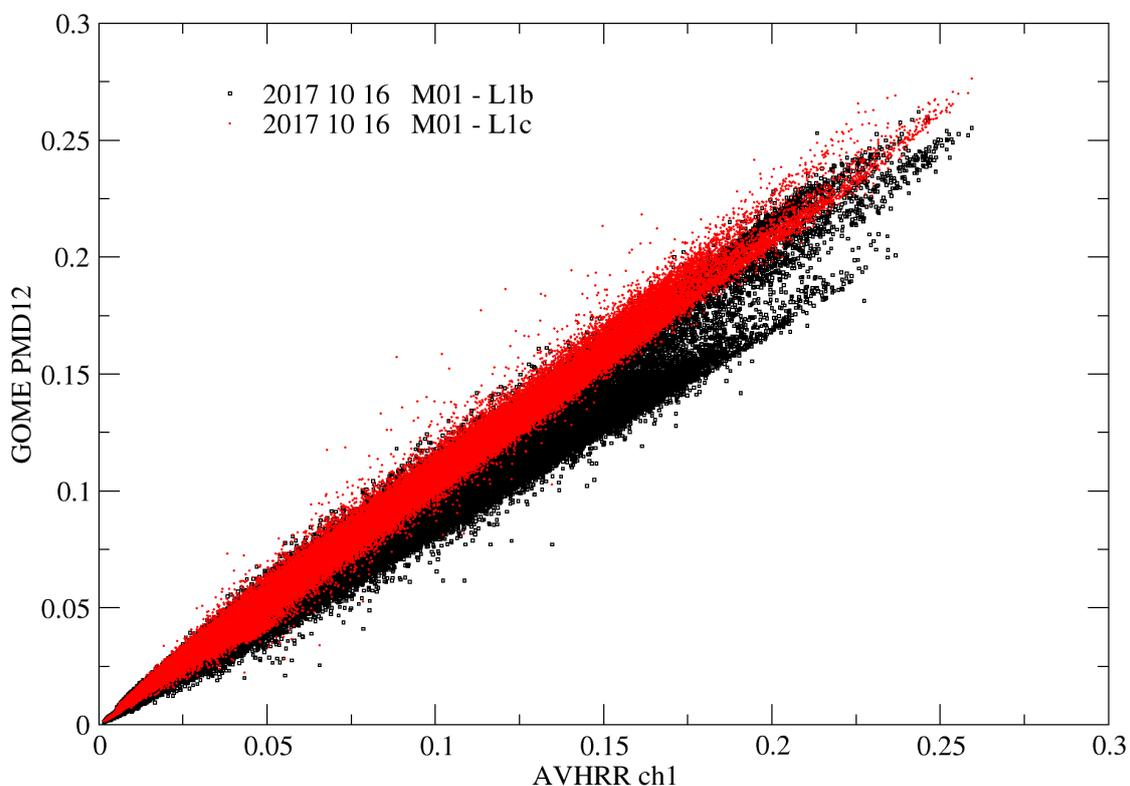
Figure 3: Reflectances of PMD12 without radiometric correction (L1b) and with radiometric correction (L1c) compared to co-located AVHRR reflectances (channel 1) to PMD12.
