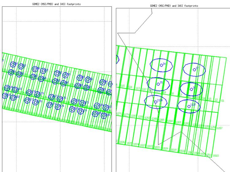
Figure 2: Schematic example for co-location of a “polygon-in-polygon” problem as used for the co-location of Metop IAS/ground pixels (blue) to GOME-2 PMD ground-pixels (green).
