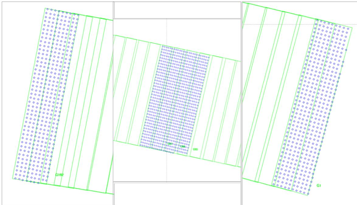
Figure 1: Schematic example for co-location of a “point-in-polygon” problem as used for the co-location of Metop AVHRR ground pixels (blue) to GOME-2 PMD ground-pixels (green).
