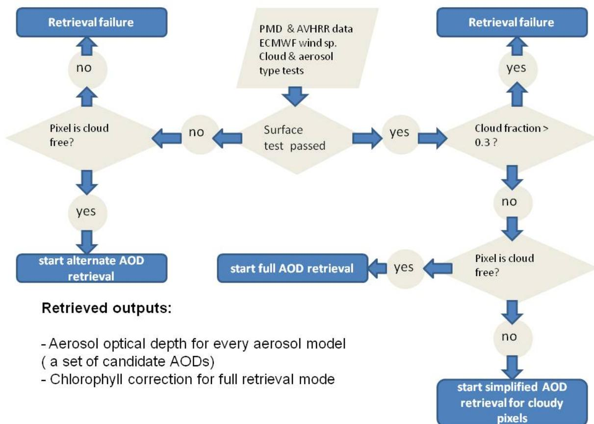
Figure 6: Retrieval algorithm selection for AOD retrieval from GOME-2. This algorithm is applied to all aerosol models provided by the LUT separately.
