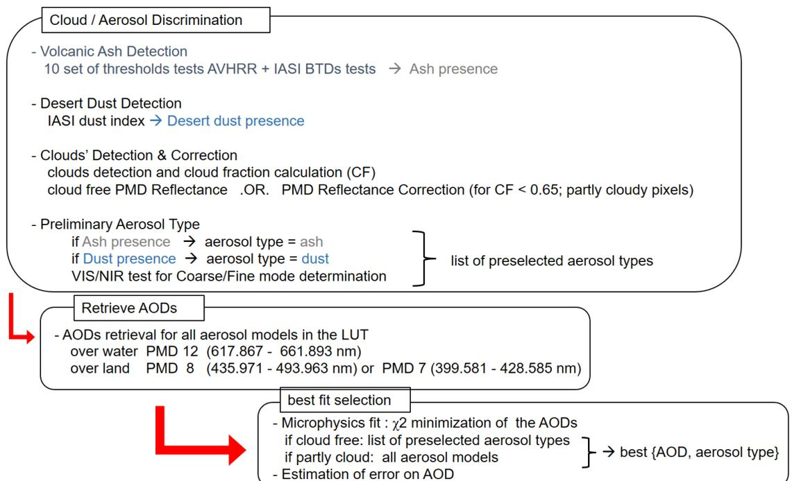
Figure 4. Flowchart of PMAp retrieval algorithm.
