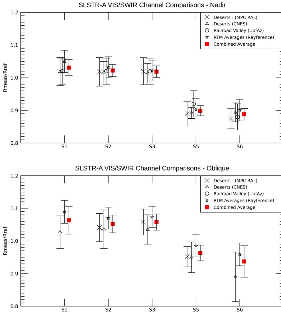
**Figure 3-1: Summary of comparisons of SLSTR VIS/SWIR channel reflectances vs. Reference methods used to provide vicarious correction factors.**
