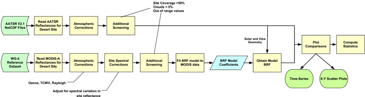
**Figure 2-1: Example of indirect comparison between two sensors (in this case AATSR and MODIS AQUA)**
