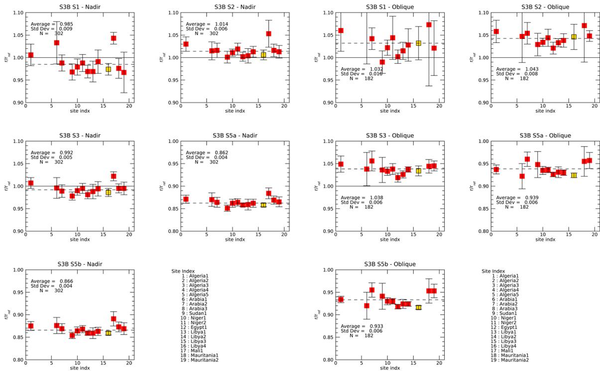
**Figure 2-3: Results of comparisons between SLSTR-B nadir and oblique views and AATSR top-of-atmosphere reflectances for each desert site. The results presented in the box are the weighted averages of all the sites, the standard-deviation and the number of measurements used in the average. The results for Libya-4 are highlighted in yellow.**
