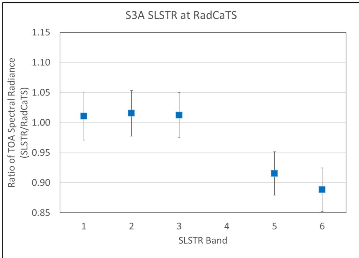
**Figure 2-4: Results of comparisons of SLSTR TOA radiances compared with data derived from in-situ measurements at Railroad Valley Playa [7].**
