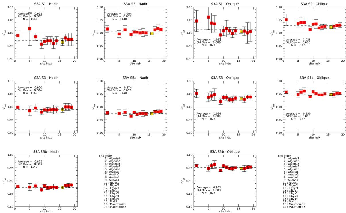
**Figure 2-2: Results of comparisons between SLSTR-A nadir and oblique views and AATSR top-of-atmosphere reflectances for each desert site. The results presented in the box are the weighted averages of all the sites, the standard-deviation and the number of measurements used in the average. The results for Libya-4 are highlighted in yellow.**
