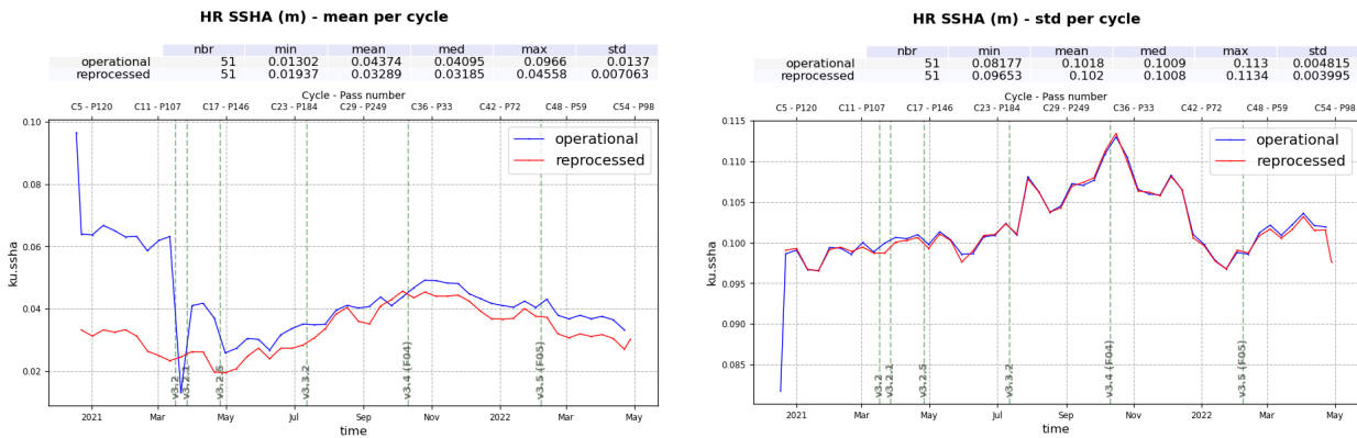
Figure 51 – Time monitoring of Sentinel-6A SSHA in meters, before reprocessing (blue) and after reprocessing (red). Left: mean per cycle, Right: standard deviation per cycle
