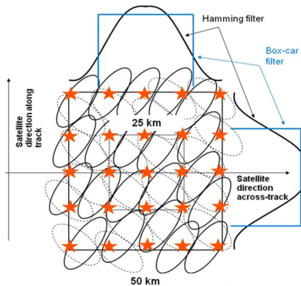
*Figure 4-5: Ground geometry of the across-track component of the spatial smoothing for  $\sigma_0$  values corresponding to two across-track adjacent nodes*
