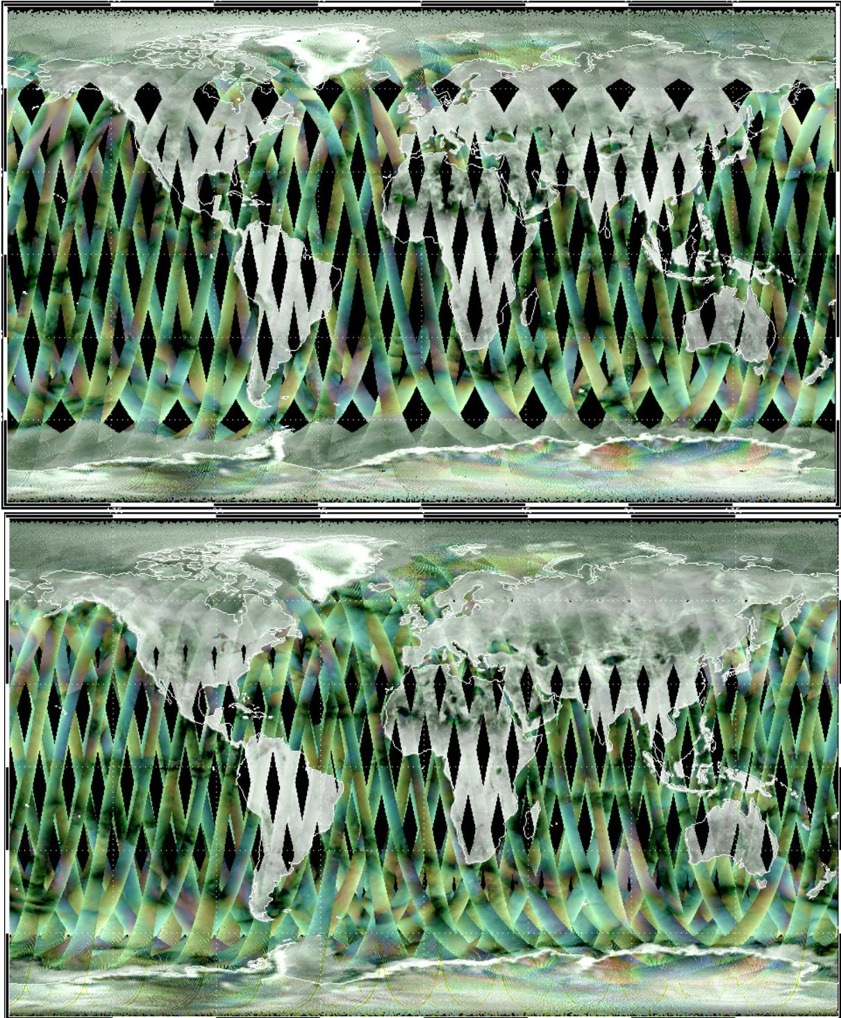
*Figure 4-2: Example of ASCAT swath coverage for 1 day, from top to bottom: Global coverage of ASCAT-A; global coverage of ASCAT-A and ASCAT-B. The values mapped are an RGB composition of the NRCS data from the FORE (Red), MID (Green) and AFT (Blue) beams.*
