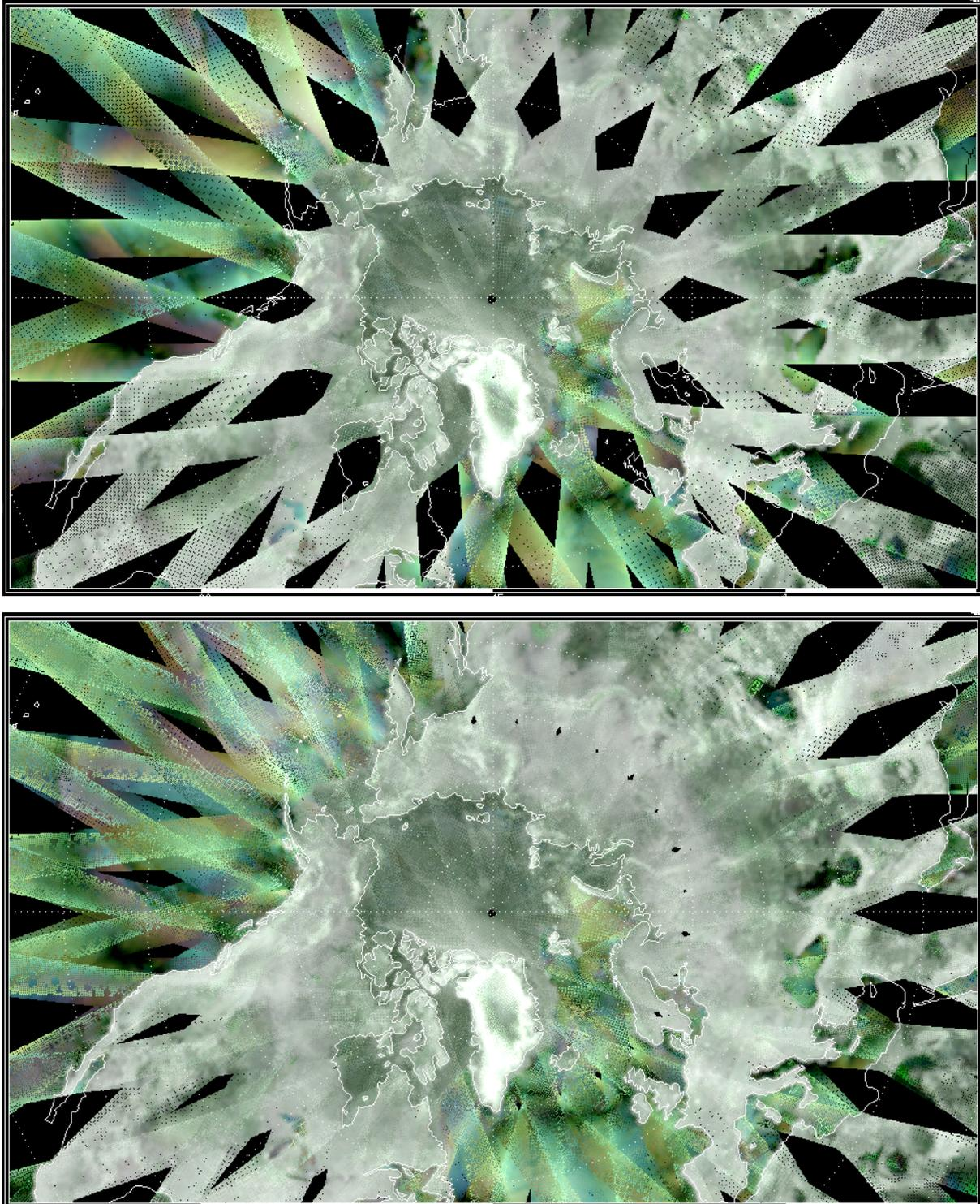
*Figure 4-3: Example of ASCAT swath coverage for 1 day, from top to bottom: Coverage over high latitudes of ASCAT-A; Coverage over high latitudes of ASCAT-A and ASCAT-B. The values mapped are an RGB composition of the NRCS data from the FORE (Red), MID (Green) and AFT (Blue) beams.*
