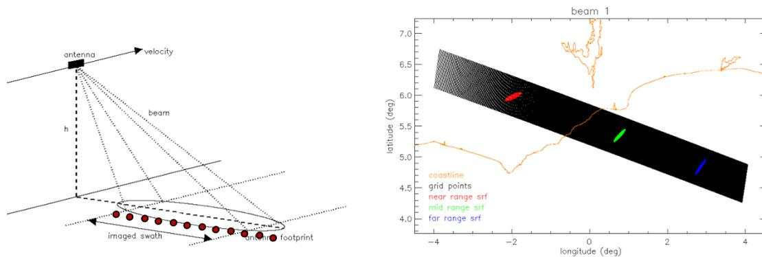
Figure 4-6: Ground geometry of the across-track component of the spatial smoothing for  $\sigma_0$  values corresponding to two across-track adjacent nodes
