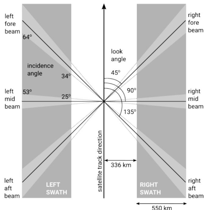
Figure 4-1: ASCAT swath geometry for a Metop minimum orbit height (822 km)
