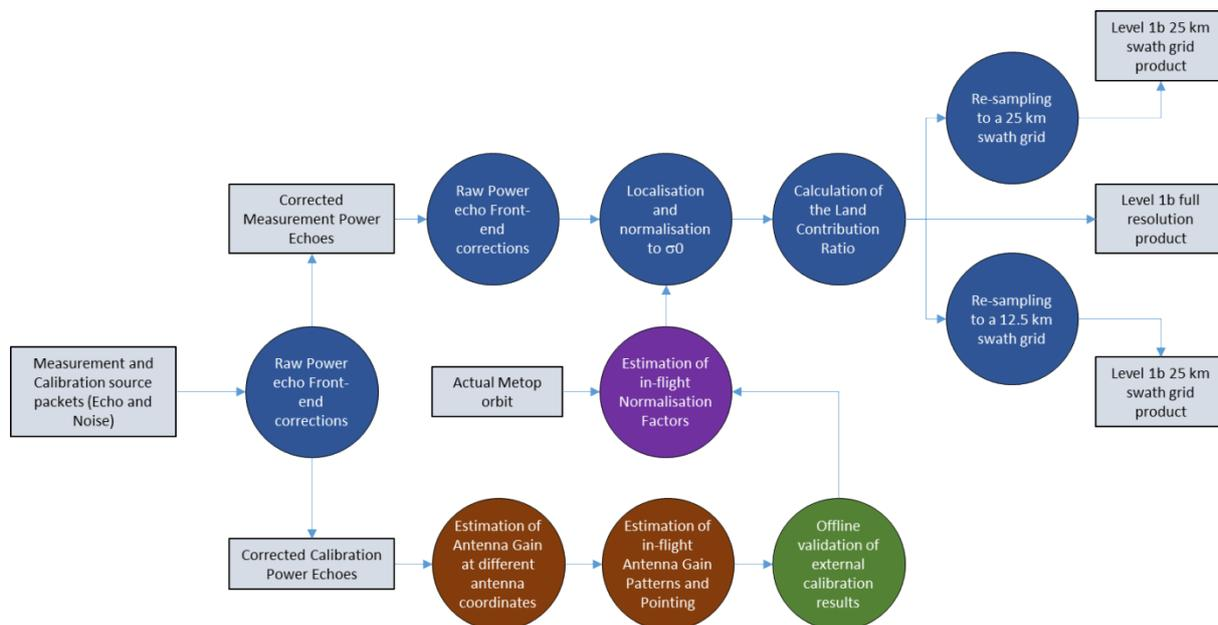
Figure 4-4: Functional overview of the ASCAT Level 1 ground processing chain.
