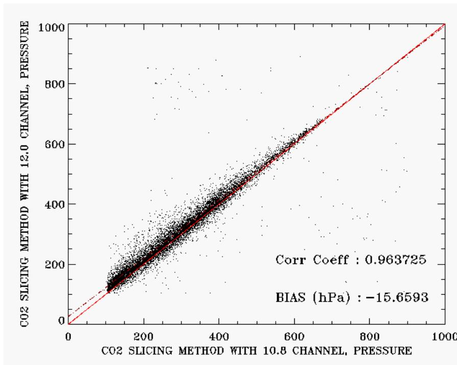
**Figure 1: Pressure calculated by CO2 slicing method using channel 10.8  $\mu\text{m}$  and 12  $\mu\text{m}$ , versus the pressure calculated by the CO2 slicing method using only the channel 10.8  $\mu\text{m}$ . SEVIRI data from the 29 March 2004 1200 UTC.**
