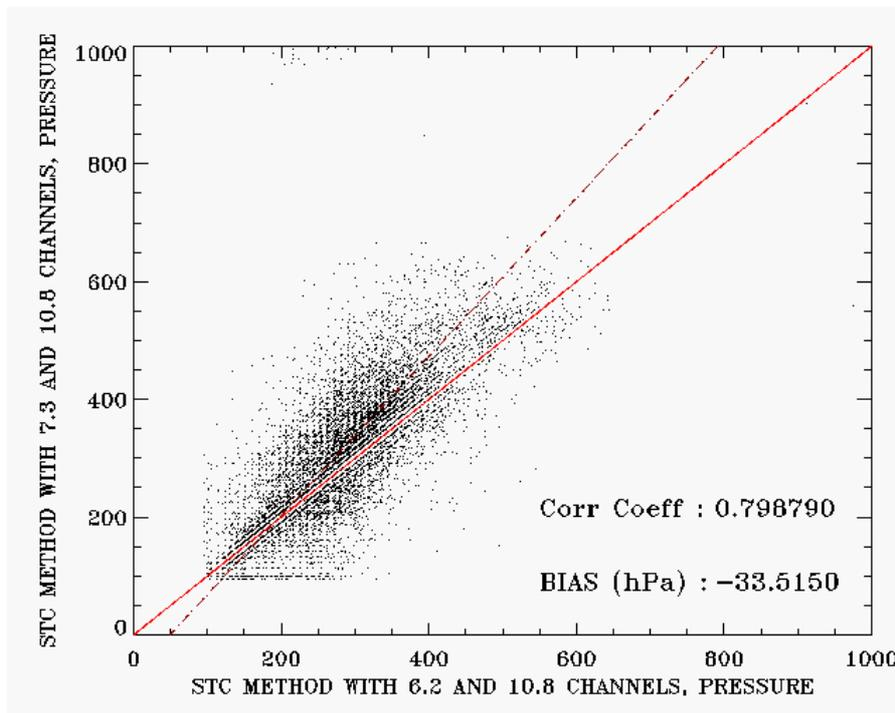
**Figure 2: Pressure calculated by STC method using channel 10.8  $\mu\text{m}$  and 7.3  $\mu\text{m}$ , versus the pressure calculated by the STC method using the channel 10.8  $\mu\text{m}$  and 6.2  $\mu\text{m}$ . SEVIRI data from the 29 March 2004 12 00 UTC.**
