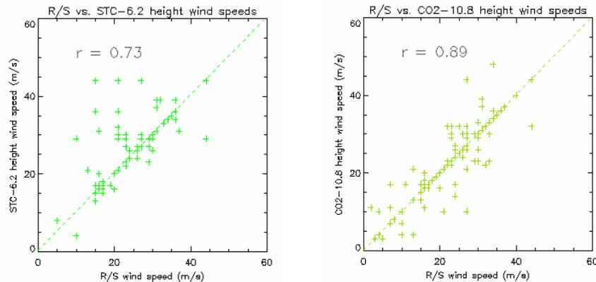
**Figure 8. Collocations between radiosonde wind speeds (horizontal axis) and IR 10.8 Meteosat 8 wind speeds at the following atmospheric levels: (left) STC 6.2 height, and (right) CO<sub>2</sub> 10.8 height.**
