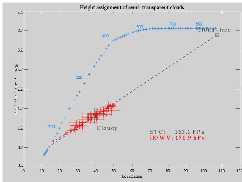
**Figure 1. Height assignment with the semi-transparency correction (STC) method and the infrared water-vapour ratioing (IR/WV) method.**
