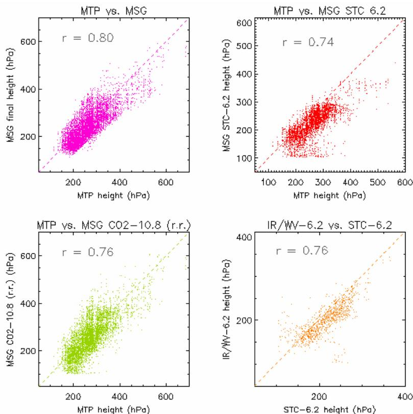
**Figure 4. Collocations between Meteosat 7 heights (horizontal axis) and Meteosat 8 heights for semi-transparent clouds, derived from IR 10.8 channel images.**
