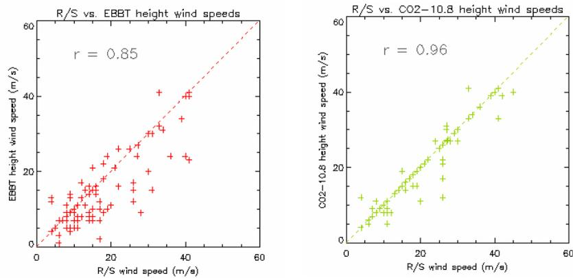
**Figure 7. Collocations between radiosonde wind speeds (horizontal axis) and VIS 0.8 Meteosat 8 wind speeds at the following atmospheric levels: (left) EBBT height, and (right) CO<sub>2</sub> 10.8 height.**
