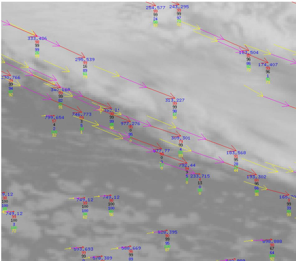
Figure 1. Three components, and for the last component (red) also the assigned pressure (with three decimals!), the quality indicator (red) and the returned values for some of the contributing AQC tests.
