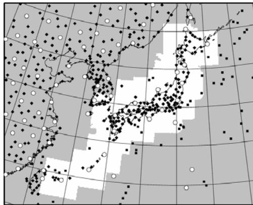
**Fig. 1 Domain of MSM. Open circle shows upper air soundings, closed symbol shows surface observations, and unshaded area shows the coverage of Radar-AMeDAS rainfall observation**
