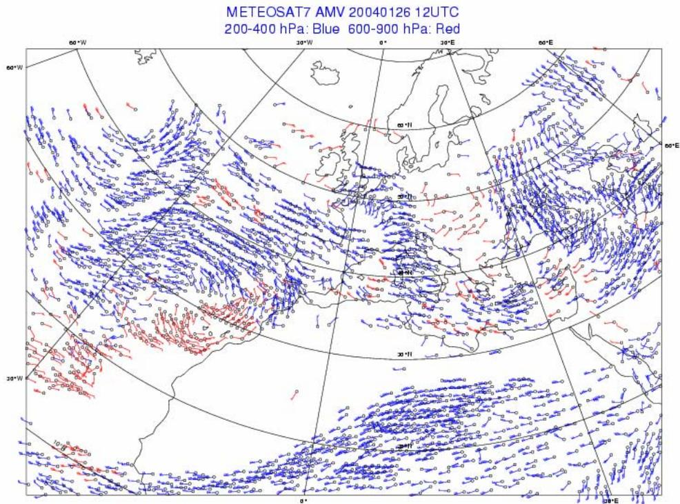
**Figure 3: Example of METEOSAT 7 AMVs in the upper (blue) and lower (red) troposphere from High Resolution Water Vapour and Visible channels over the CNMCA Regional NWP system domain.**
