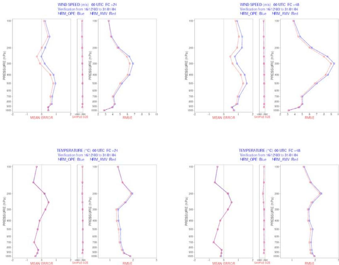
**Figure 6: Wind speed and temperature mean error and wind vector and temperature RMSE of EURO-HRM t+24, t+48h forecasts from CNMCA 3DVar analysis with (red) and without (blue) the ingestion of Meteosat 5 and 7 AMV data verified against European RAOB observations.**
