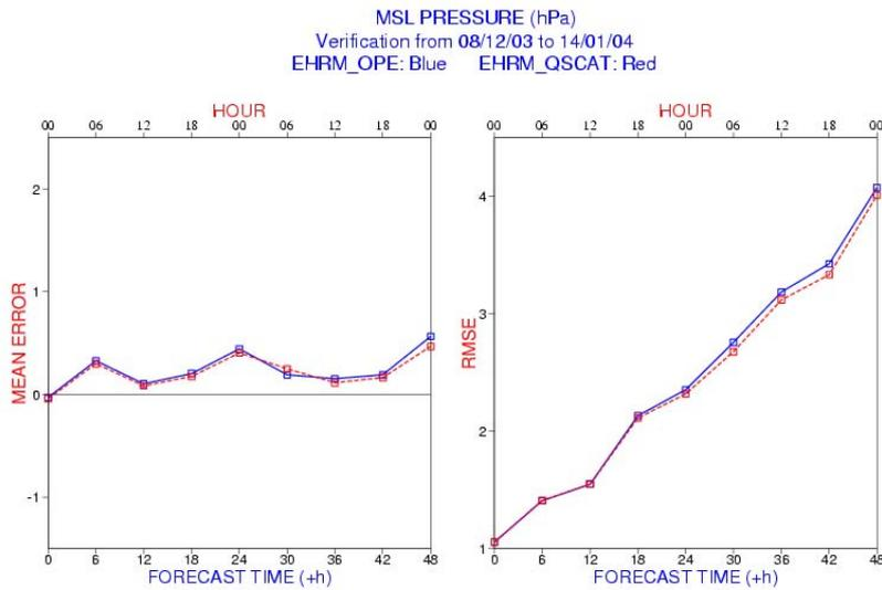
**Figure 5: Mean errors and RMSE of EURO-HRM MSL pressure forecasts from CNMCA 3DVar analysis with (red) and without (blue) the ingestion of Quikscat retrieved winds verified against lowland SYNOP observations.**
