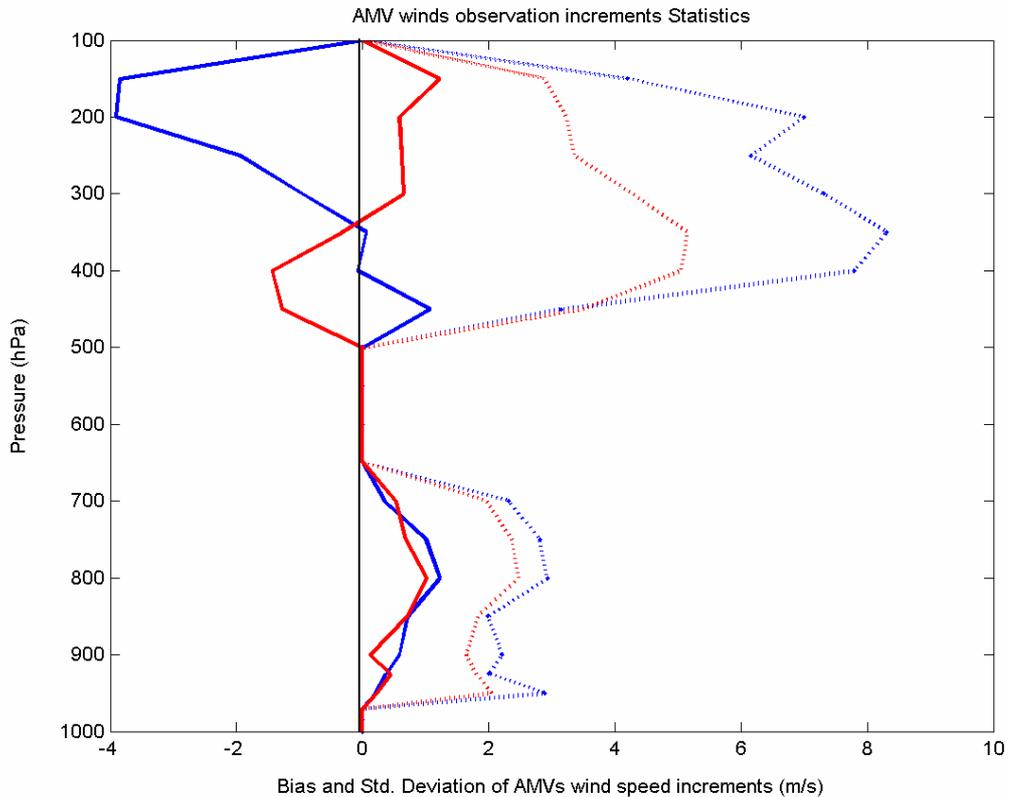
**Figure 4: AMVs wind speed bias (solid) and standard deviation (dashed) with respect to the t+6h EURO-HRM first guess field. Red lines for height adjusted observations.**
