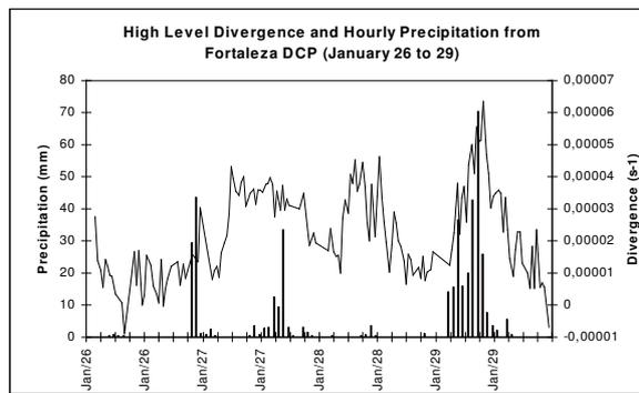
Figure 6 – High level GOES wind divergence and hourly precipitation observed by Fortaleza’s DCP for January 26 to 29
