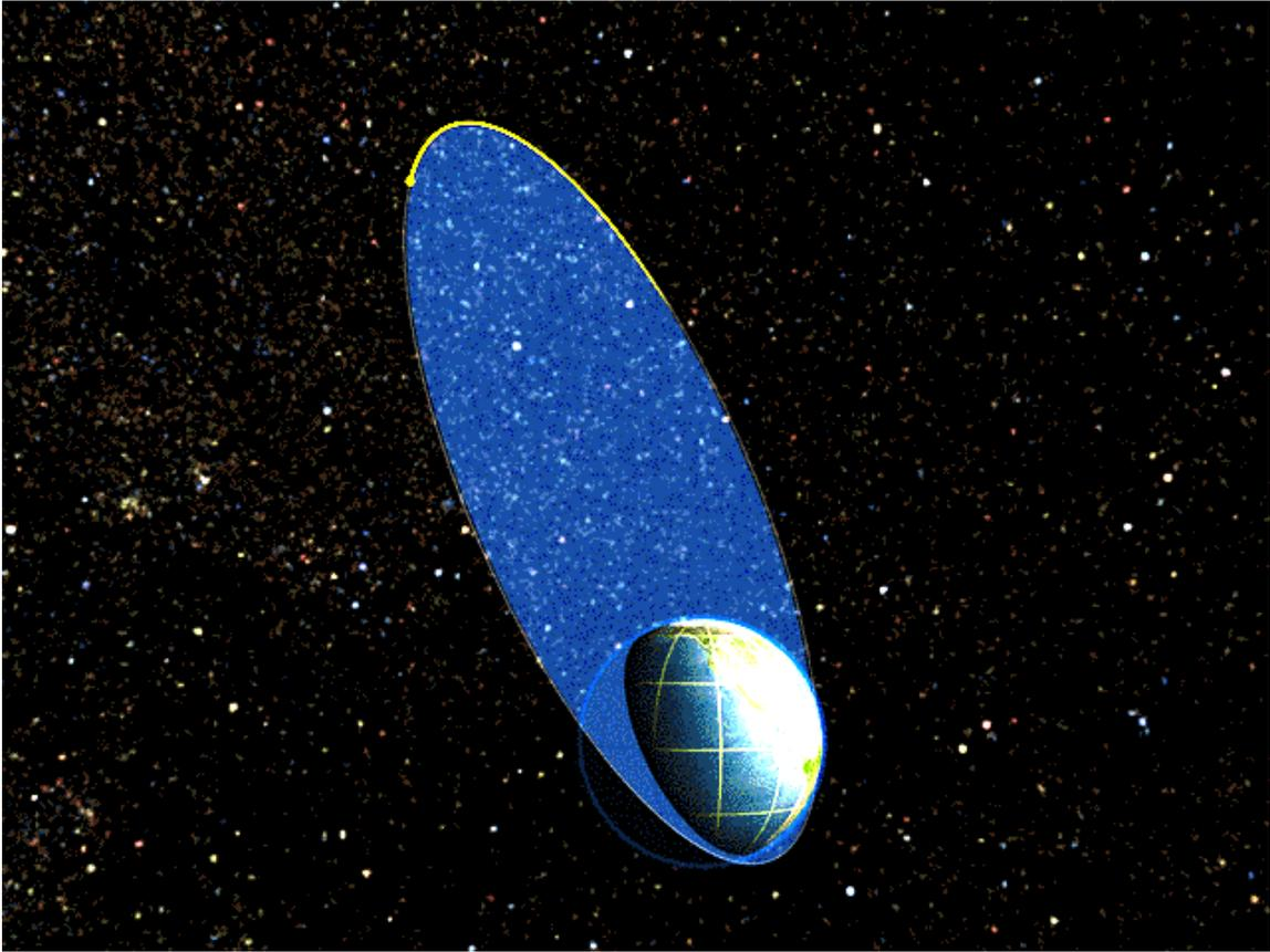
*Fig.1 The Molniya orbital plane. Due to the second Kepler Law, the satellite spends most of the time in the near-apogee part of the orbit (yellow trace), from where it will provide a quasi-stationary view of much of the northern hemisphere, including the high latitudes.*
