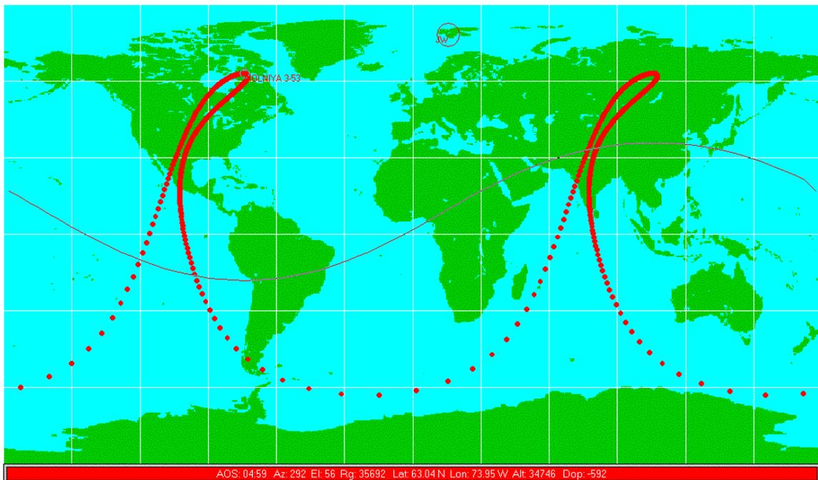
*Figure 2. Example of a near-Molniya orbit (Russian Molniya 3-53 satellite). Location plotted in red every 100 s; all areas N of solid line are visible from the western hemisphere apogee location indicated by satellite name.*
